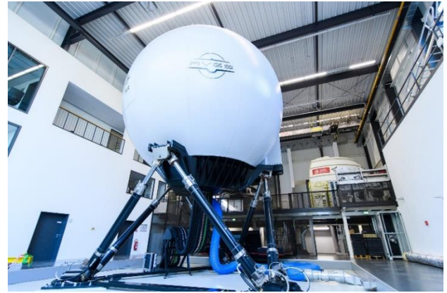
Figure 10 Air Vehicle Simulator (AVES) at DLR Braunschweig
