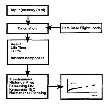
Fig. 10: Functional structure of the ground station software
