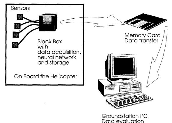
Fig. 9: Example for a system application including the ground station
