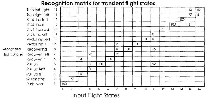
The missing flight states in this matrix are associated to steady flight states
