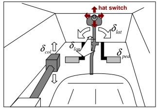
Fig. 3 Main control Inputs used by the pilot
