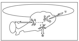
Fig. 4 Main helicopter flight dynamic parameters
