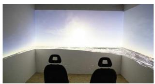
Fig. 19 PycsHel: a prototyping and simulation platform for helicopters currently in development at ONERA Salon de Provence
