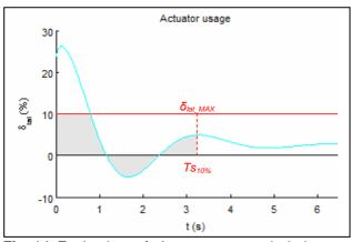
Fig. 14 Evaluation of the energy used during an attitude change simulation (model (15))
