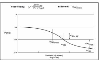
Fig. 9 Definition of small amplitude criterion parameters
