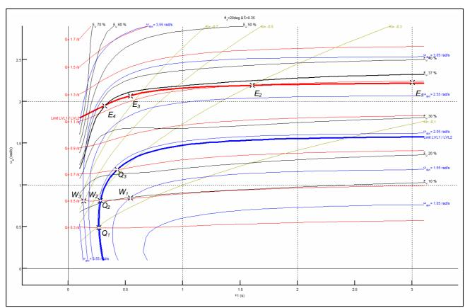
Fig. 12 Example of a chart generated for the roll axis control law of a cargo-type helicopter
