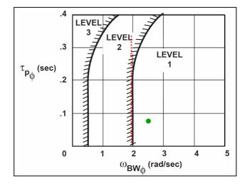
**Fig. 10** Accuracy criterion: bandwitdth / phase delay The Level 1 / Level 2 limit can be approximated by a vertical line at  $\omega_{BWphase} = 2rad/sec$  (red dotted line on **Fig. 10**). Indeed, the values of phase delay  $(\tau_p)$  seem to be mainly influenced by the natural system delays. The gains of the control laws seem to have negligible influence on its value **[10]**, for stabilized systems at least.
