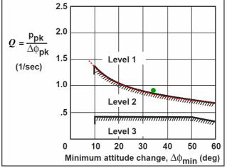
Fig. 8 Quickness criterion: attitude quickness
