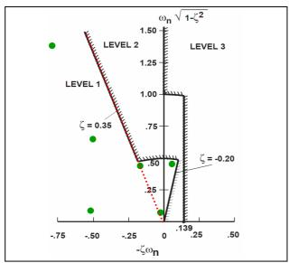
Fig. 6 Stability criterion: pole placement
