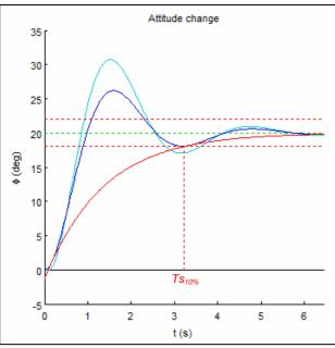
**Fig. 13** Evaluation of the approximated settling time to 10%.
