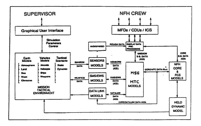
Figure 3: NH90 mission simulator functional architecture
