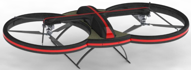
Figure 1: Electric dual-rotor VTOL configuration, courtesy of SAB Group S.R.L.
