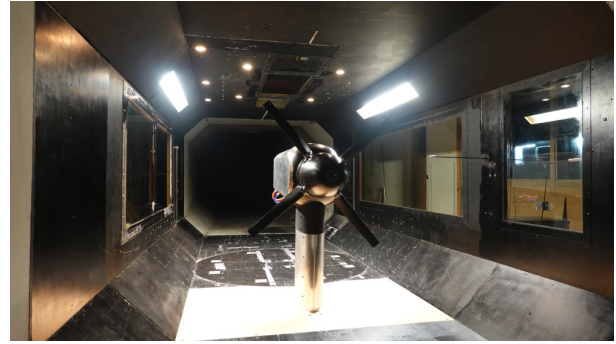
Figure 1: The UKNRR installed in the DeHavilland tunnel.
