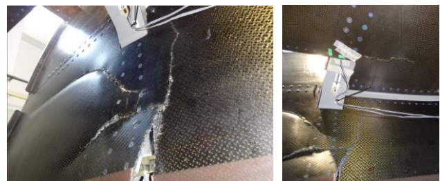
Figure 13: Stub wing after final test with rupture beyond ultimate load. View is showing transition stub wing to fuselage with rupture close to the boundary
