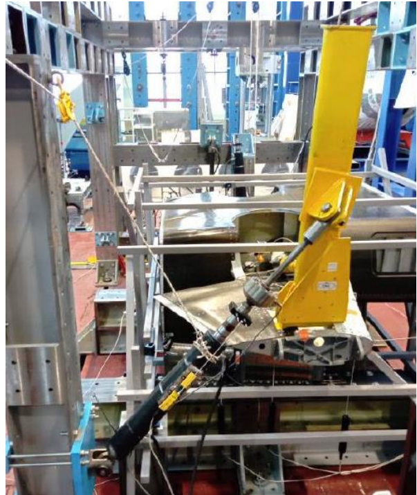
Figure 12: LH stub wing side with dummy landing gear (yellow) and hydraulic actuator installed, courtesy of INCAS & AVIATEST.
