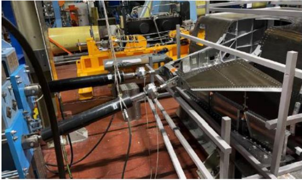
Figure 10: Actuators simulating the wing loads on the RH stub-wing, courtesy of INCAS & AVIATEST.
