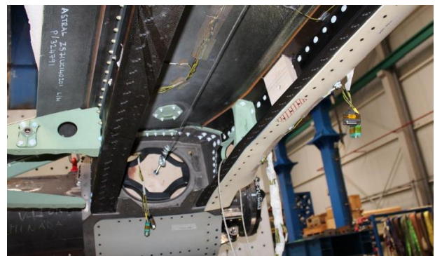
Figure 23: Tension wire representing the LDL mounted to a wooden plate in the Cradle opening
