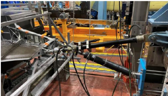
Figure 11: Actuators simulating the wing loads on the LH stub-wing, courtesy of INCAS & AVIATEST.
