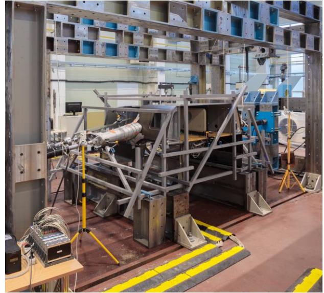
Figure 9: Basic arrangement of the stub-wing specimen in the test-rig for the wing load cases, courtesy of INCAS & AVIATEST.
