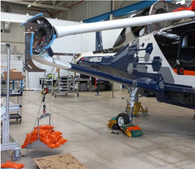
Figure 5: Example for the GFEM accuracy test on the flying demonstrator with loads applied by sand bags (in orange) at the wing tips.
