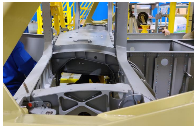
Figure 3: The stub wing region at the lower wing connection to the fuselage, with frame 4 and 5, root and end ribs (by courtesy of the Romanian consortium RoRcraft).
