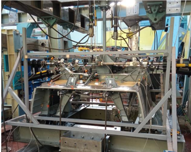
Figure 17: Set-up of the front cross beam test in the test campaign.
