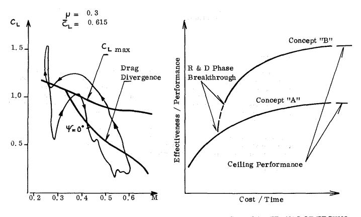
FIGURE 2 - WORKING CONDITIONS OF A ROTOR BLADE ELEMENT AT 0.71 RADIUS - REF. : 10
