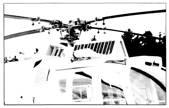
Figure 11 Photograph of Centrisep installed on MBB BO-105
