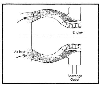
Figure 25 EIPS Dust Particle Trajectory
