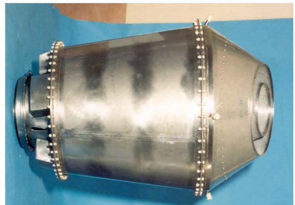
Figure #2 : Multi-duct exhaust device
