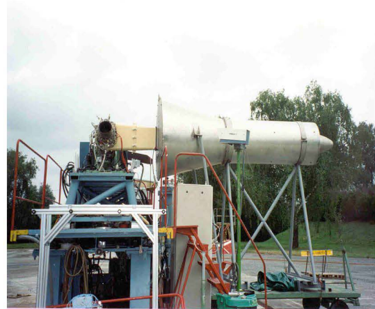
Figure #4: muffler on the air intake (exhaust noise)
