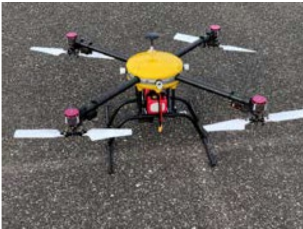
Figure 1. A quadrotor drone with variable pitch controls [4]
