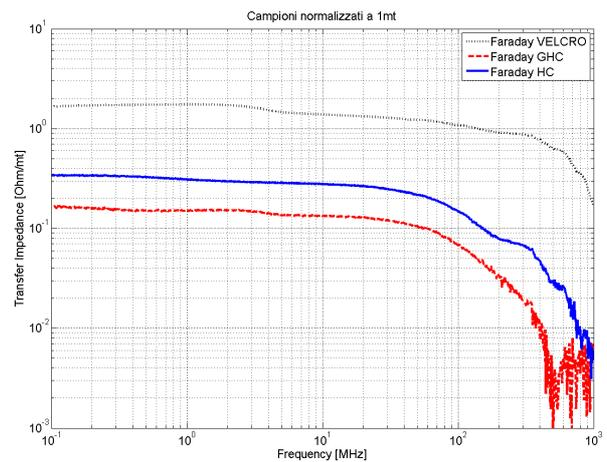
Figure 8- Transfer Impedance from (TI) CashFlex
