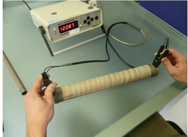
Figure 2 - The DC measurement offer just a view in Ohm
