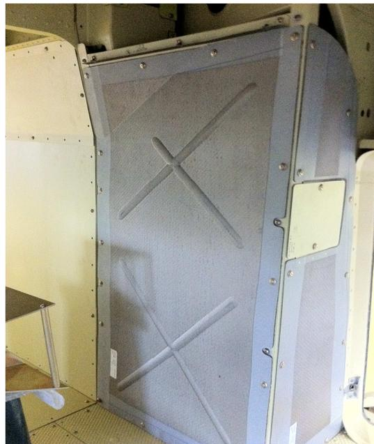
Figure 10 - Fig 10 panel in thermoplastic resin with carbon and conductive fabric
