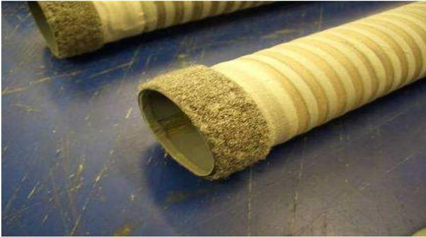
Figure 4 - Connection with Velcro conductive
