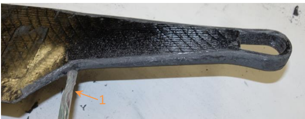
Figure 49: Blade neck with blade neck caps
