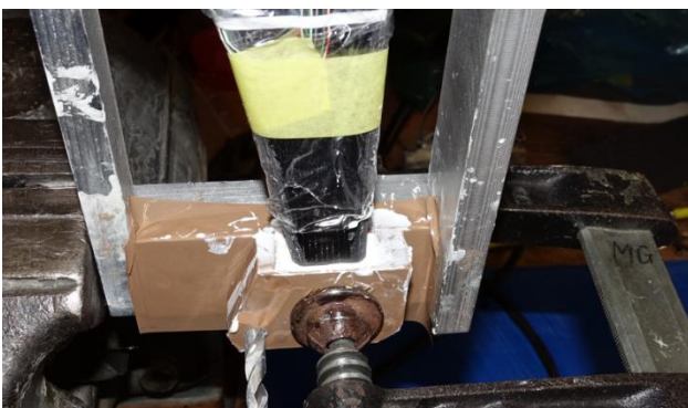
Figure 50: Blade shoe mounting
