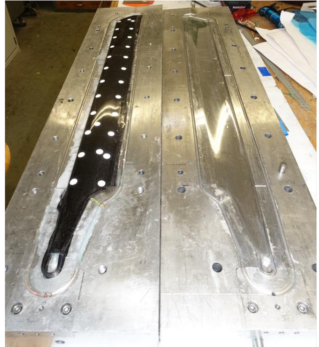
Figure 46: Rotor blade in the lower mold
