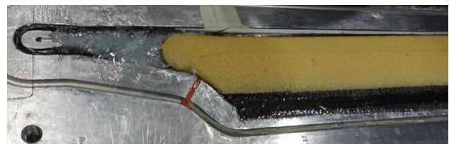
Figure 43: Bottom shell final preparation before assembly
