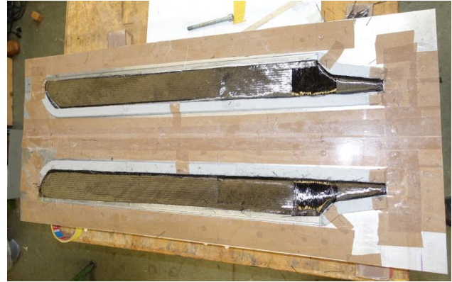
Figure 12: Mold halves with fiber material
