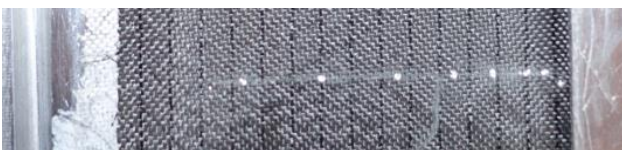
Figure 21: Upper blade skin with sensor holes
