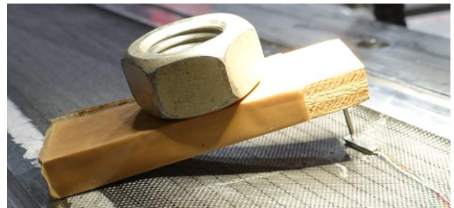
Figure 22: Gluing in a pressure sensor
