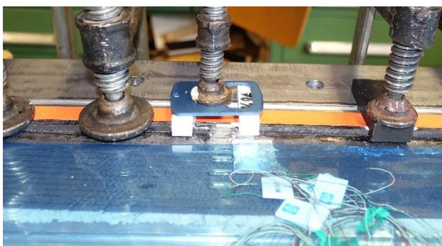
Figure 27: Gluing in the nose mass cap
