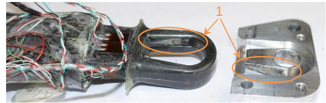
Figure 54: Blade root and shoe inspection
