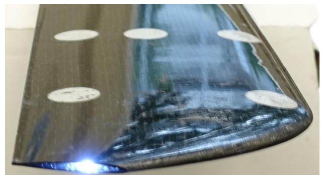
Figure 56: Blade tip with LED
