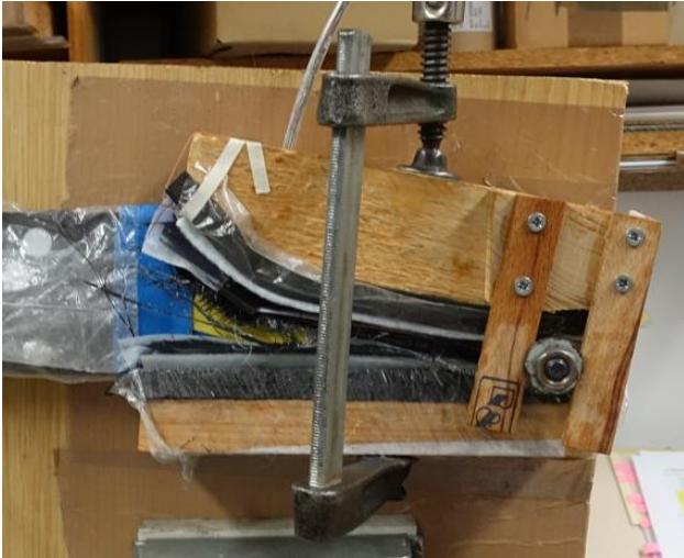
Figure 48: Pressing on the blade neck cap layers
