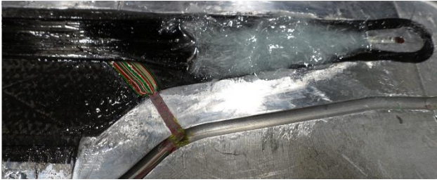
Figure 44: Upper skin with thickened resin
