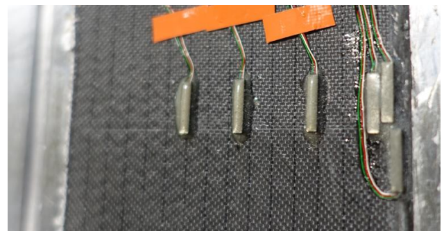
Figure 24: Pressure sensors inside the lower skin
