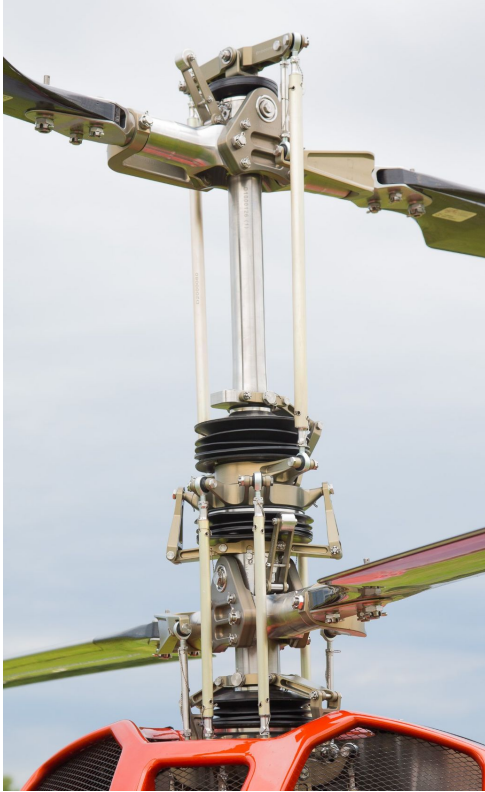
Figure 3: The rotor system of the flight demonstrator
