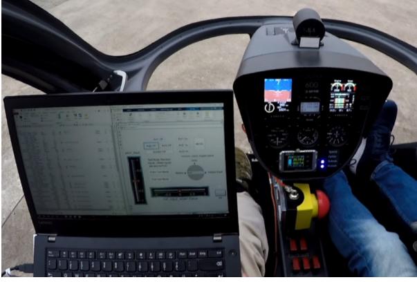
Figure 33: Failure simulation through laptop interface in the tethered flight demonstrator
