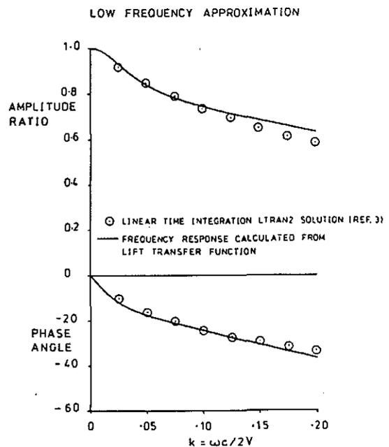
FIG. 2. PLUNGE FREQUENCY RESPONSE,  $M=0.8$ .
