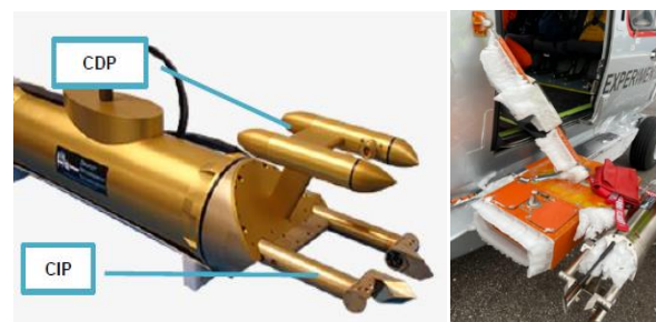
Figure 9: Cloud Combination Probe – CCP – installed on H175B
