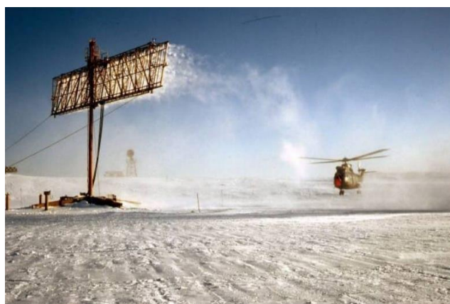
Figure 5: Puma icing test at the NRC Spray Rig, in Ottawa, Canada.
