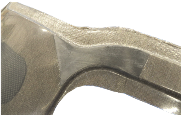
Figure 17: Carbon fiber reinforcement of critical load path at outer shell of cabin door B after demolding
