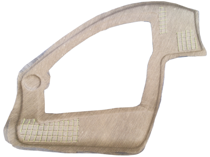
Figure 18: PowerRib™ reinforcement of door D outer shell during layup
