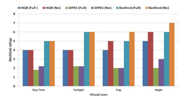
Figure 13: Motion cueing effects on pilots' workload and handling quality ratings in day, twilight, fog and night visual environments, green 45 airwake at wind speed of 30 kts, sea state 5.
