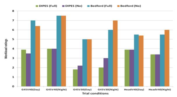
Figure 12: Motion cueing effects on the averaged pilots' workload ratings in day and night visual environments, sea state 5 (Trial conditions: G45: green 45 airwake; Head: headwind airwake; V40/30: wind speed 40/30 kts).
