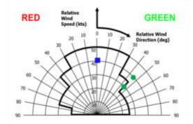
Figure 1: Ship-Helicopter Operating Limits (SHOL) diagram obtained in the Liverpool flight simulator [4]. The square and circular marks indicate the test points in this study.
