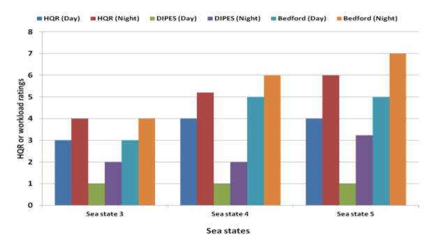
Figure 11: Bar plots of the workload and handling quality ratings in day and night visual environments of the lateral reposition task, green 45 airwake at wind speed of 30 kts, sea state 3, 4 and 5.
