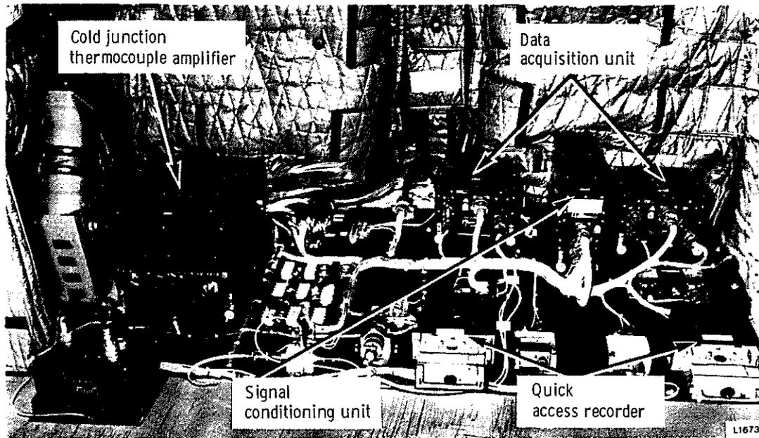
Fig.6. Rear view of cabin showing equipment and recorders on baseboard
