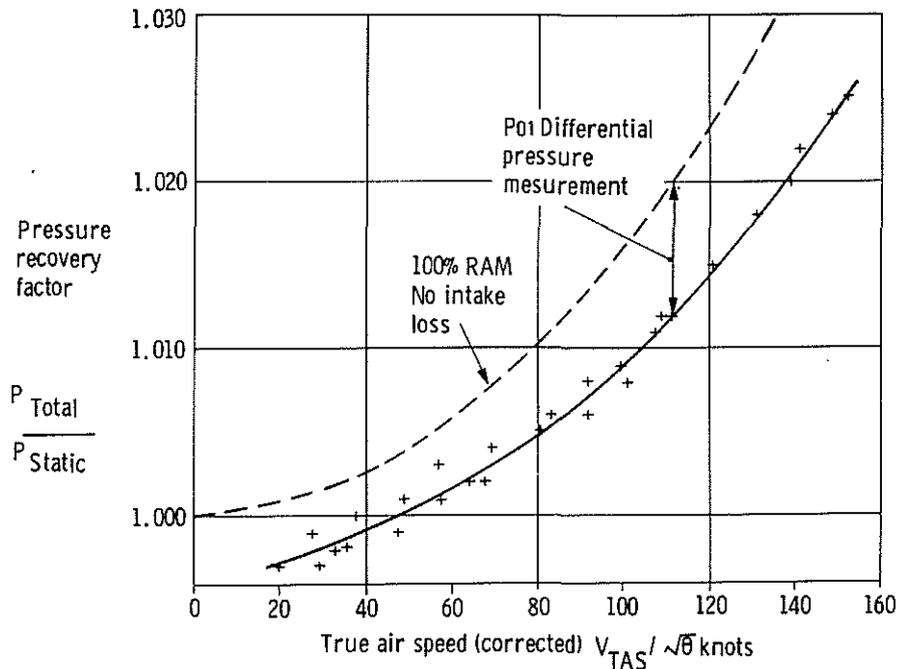
Fig.9. Intake pressure recovery
