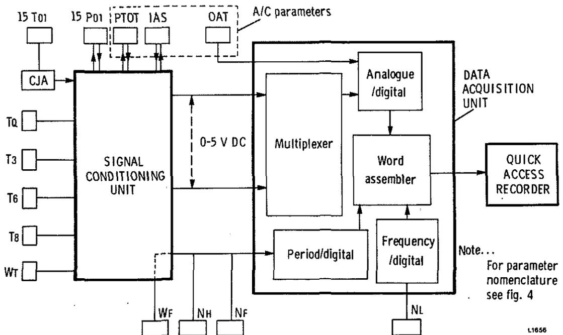
Fig.5. Measurement system used to assess installed engine power
