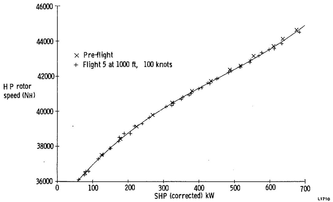
Fig.11 Comparison of critical measurements taken on the test-bed and during flight trials
