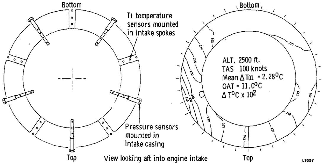
Fig.7a Position of temperature and pressure sensors in Gem engine intake
