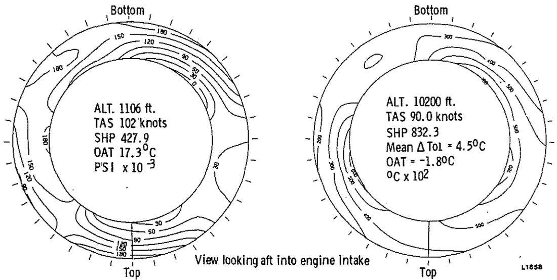
Fig.7c Typical intake pressure profile
