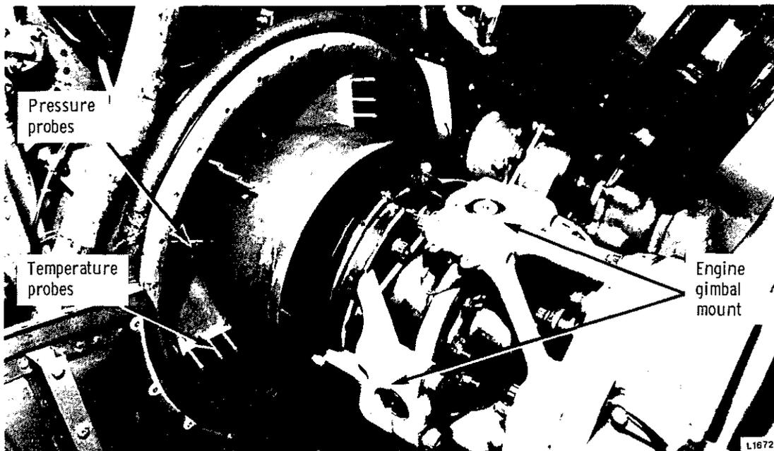
Fig.1. Plate showing relative position of the pressure and temperature probes in the engine air-intake
