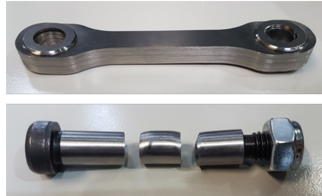
Fig. 17: Centrifugal force tensile strength test of the metal stack
