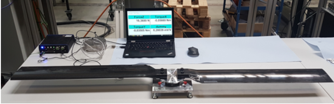
Fig. 6: MERIT rotor blade balancing
