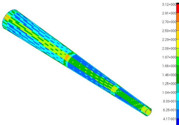
**Figure 14 Thickness distribution of tail boom**
