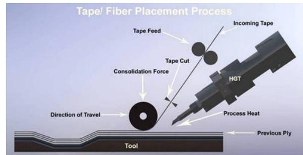
**Figure 1 Fiber placement process (photo courtesy of Automated Dynamics)**
