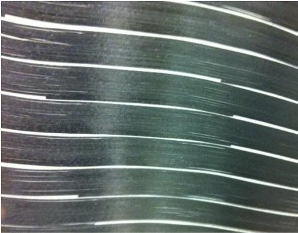
**Figure 10 0% overlap ratio ply lay-up**
