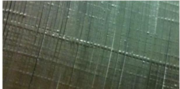
Figure 7 Local Fiber Buckling
