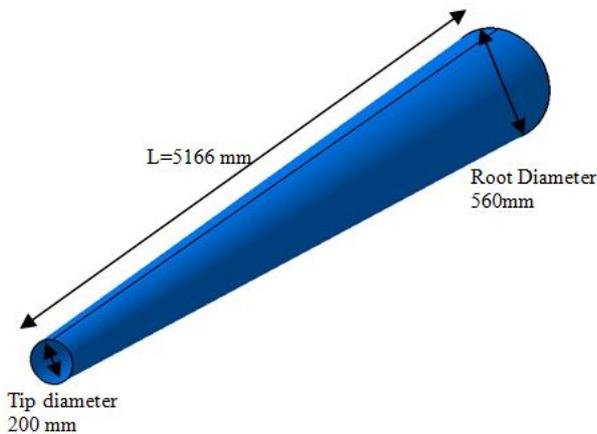
**Figure 4 Conical shell dimension**
