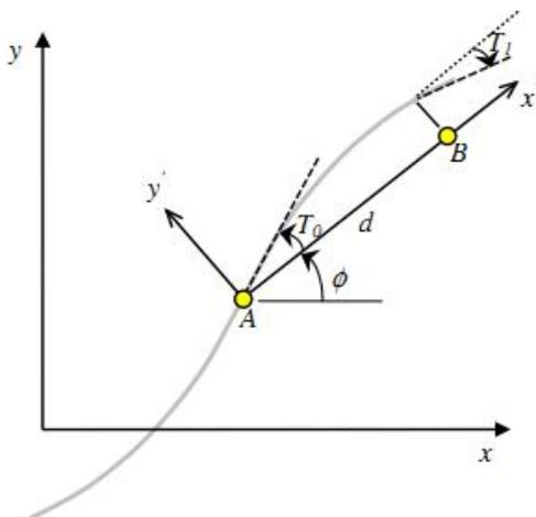
Figure 2 Fiber path parameters
