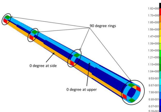
**Figure 13 Thickness distribution**
