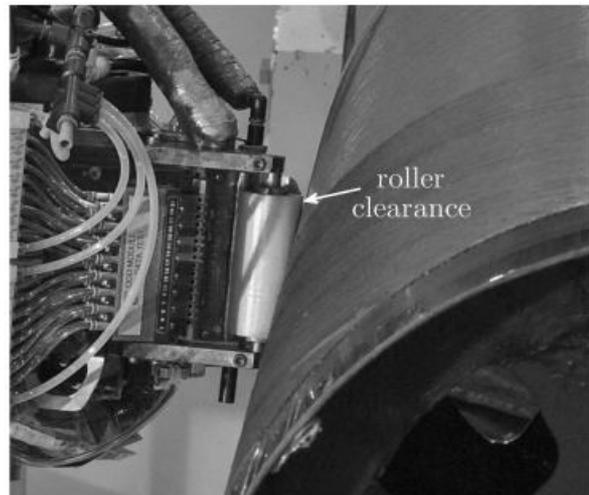
**Figure 12 Roller clearance on cylinder surface [1]**
