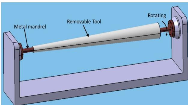
**Figure 11 Mandrel for manufacturing of tail boom**
