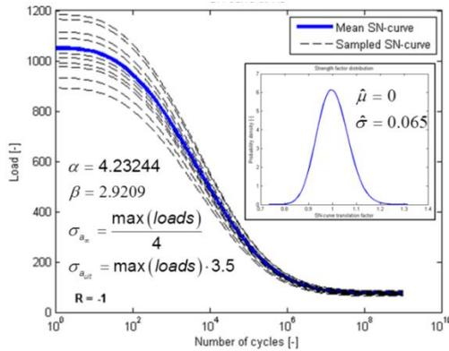
Figure 5.1: Definition the S-N-P curve in the reference problem. See also equations (2.1) and (2.5). “Loads” refers to all sampled load signals, as in Figure 5.2.
