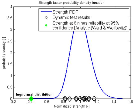
Figure 2.2: Exemplary fatigue test results (normalized by the MLE S-N curve), the derived MLE estimate of the PDF of normalized fatigue strength ( $SF$ ), and the strength factor corresponding to the conservative working curve.
