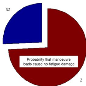
Figure 4.1: Pie chart showing how probable it is that there are load cycles within a particular manoeuvre above the endurance limit (Z) or not (NZ).
