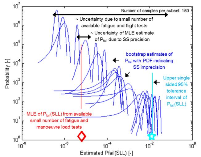
Figure 4.8: Example of the PDFs of bootstrap estimates of  $P_{fail}(SLL)$ . The width of a PDF represents uncertainty due to limited SS accuracy and the variance in the mean of the different PDFs represents uncertainty due a low number of fatigue and manoeuvre load tests. It demonstrates that imprecision from SS is small with respect to uncertainty due to a low number of fatigue and manoeuvre load tests. (Result for seven available fatigue tests and fifteen instances per manoeuvre)
