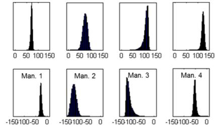
Figure 5.3: Example of reference flight regime maximum (above) and minimum (below) load (marginal) distributions
