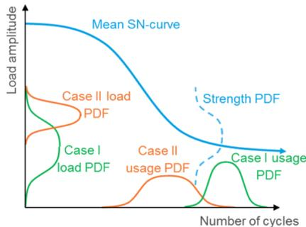
Figure 3.1: Schematic of the random model framework for recent (semi-)analytical SLL reliability models (shown with two load cases).
