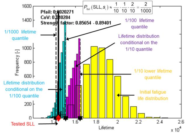
Figure 4.4: Example of Subset Simulation where it takes three intermediate failure events (black stars) to reach the SLL under evaluation (red diamond). The initial lifetime sample is in yellow, the lifetime distribution conditional on  $F_1$  is purple and the lifetime distribution conditional on  $F_2$  is light blue.  $P_{fail}(SLL, s_i) \approx 0.1 \cdot 0.1 \cdot 0.2 = 0.002$
