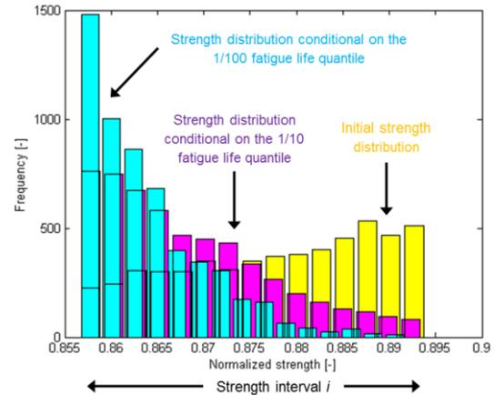
Figure 4.5: Strength samples from SS from the example in Figure 4.4. Note that the strength generally decreases as the intermediate failure events become less probable.
