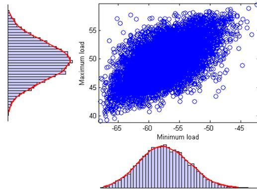
Figure 4.2: A large sample from a fitted multivariate flight regime minimum and maximum load distribution. (i.e. manoeuvre damage is zero) The corresponding marginal distributions are also shown.
