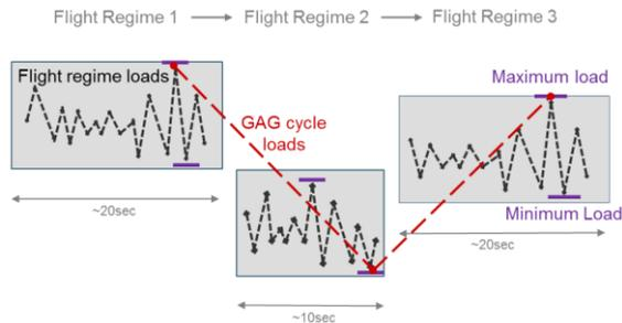
Figure 2.3: Manoeuvre (flight regime) loads and Ground-Air-Ground loads. These loads together make out the full load spectrum.
