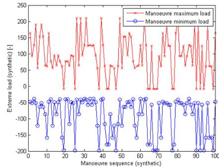
Figure 5.5: Example of sampled GAG extreme manoeuvre loads before extreme load and PV-filtering.
