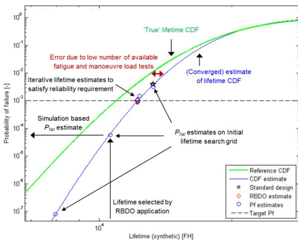
Figure 5.11: Illustrative result from a custom developed RBDO application to predict fatigue life using the simulation-based fatigue life substantiation model. Note that  $P_{fail}$  estimates around the same lifetime do not differ much, demonstrating the high precision of SS in the newly proposed method (i.e. with 150 samples per subset).
