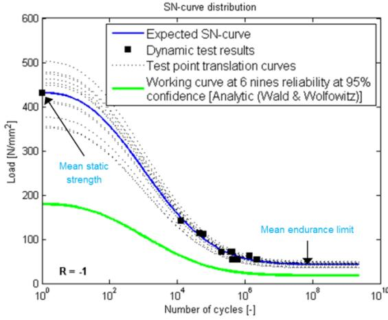
Figure 2.1: Example of constant amplitude fatigue test results, the MLE S-N curve and conservative working curve for a component from the dynamic system.
