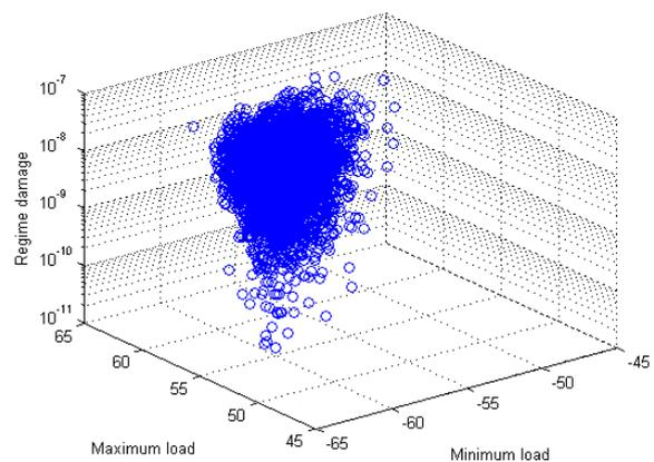
Figure 4.3: A large sample from a fitted multivariate flight regime damage and extreme load distribution.
