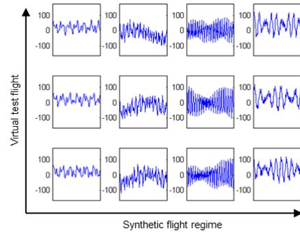
Figure 5.2: Example of artificially generated test flight data. Note the similarity between samples for the same regime and the difference between the regimes.
