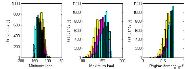
Figure 4.6: SS samples of the minimum load, maximum load and regime damage of a flight regime from the example in Figure 4.4. Note that, for example, the maximum load (middle) generally increases with less likely intermediate failure events, as would be expected.
