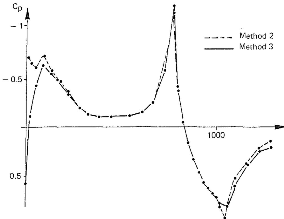
Fig. 4 — Pressure distributions on lower symmetry line without wake.
