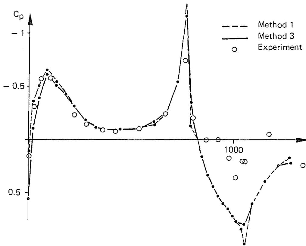
Fig. 5 — Pressure distributions on lower symmetry line without wake.
