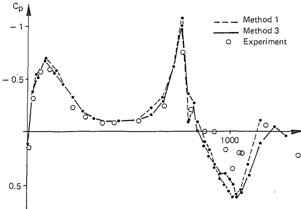
Fig. 6 — Pressure distributions on lower symmetry line with wake.
