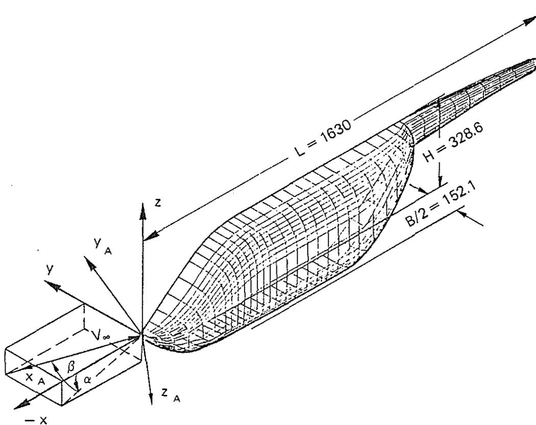
Fig. 2 — Geometry of the helicopter model fuselage.
