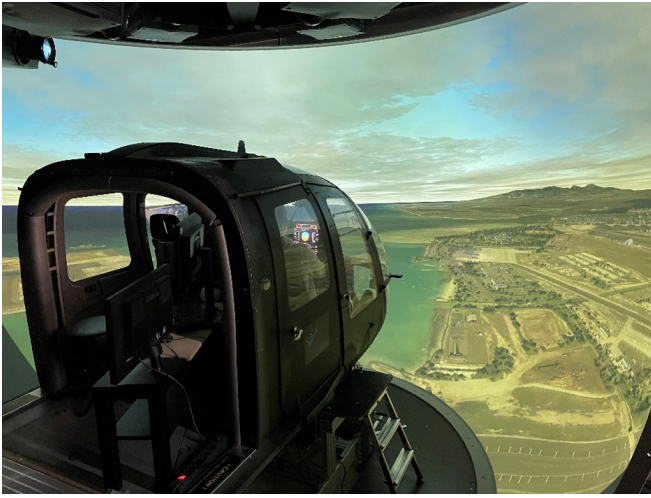
Figure 5: ROSIE X flight simulator at the Institute of Rotorcraft and Vertical Flight at Technical University of Munich
