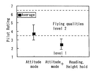
Figure.15 Pilot Rating of Law-speed flight task in IMC with and without Hold Function
