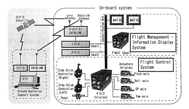
Figure.1 Configuration of the on-board system
