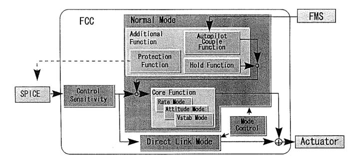
Figure.3 Function block diagram of the flight control law
