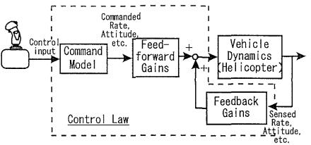
Figure.4 Configuration of the Core Function
