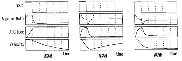
Figure.5 Control response of each response type in Core Function
