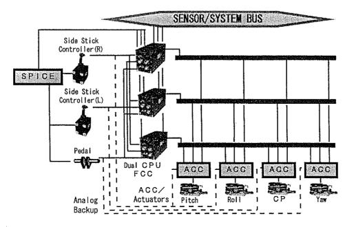
Figure.2 Coniguration of the flight control system
