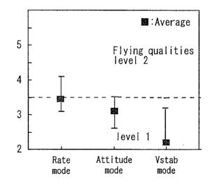
Figure.14 Pilot Rating of Low-speed climb and descent in VMC
