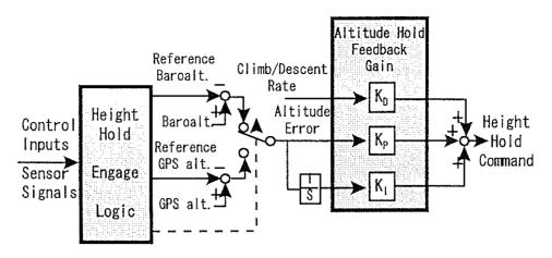
Figure.6 Block diagram of Hold Function
