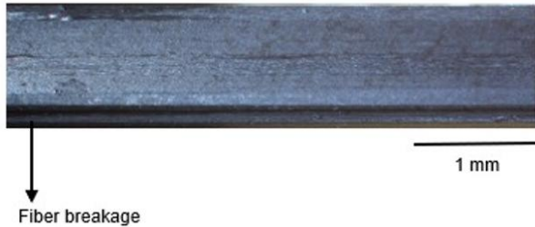
Figure 5: Optical image of unconditioned coupon completing 10^6 cycles at 50% load level.
