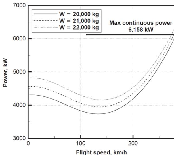
Fig. 9: Typical power versus speed curve for a Boeing CH-47 [18, p. 376]
