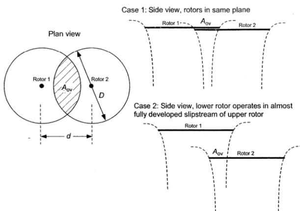
**Fig. 12: Hover condition for a tandem system with stream tube around the two rotor disks [19, p. 107]**
