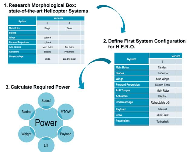
**Fig. 8: Pankl Aerospace's approach to generate the first basic system configuration and power calculation for H.E.R.O.**
