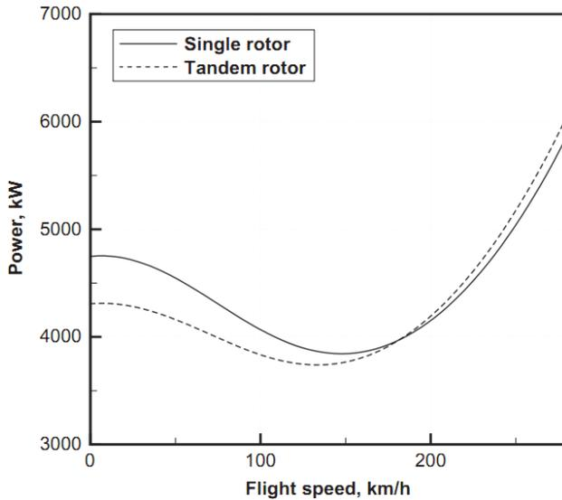
**Fig. 17: Comparison of power versus speed diagrams for a single and tandem helicopter with the same weight [18, p. 379]**
