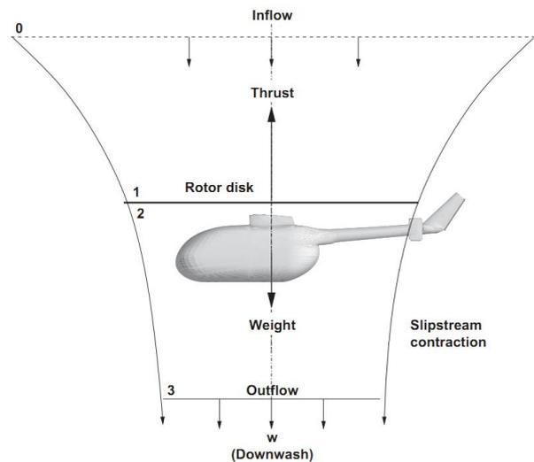
Fig. 10: Hover condition with stream tube around the rotor disk and airframe [18, p. 316]
