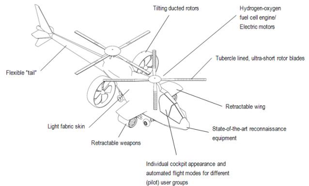
**Fig. 4: Core features of Pankl Aerospace's vertical flight aircraft concept "H.E.R.O."**
