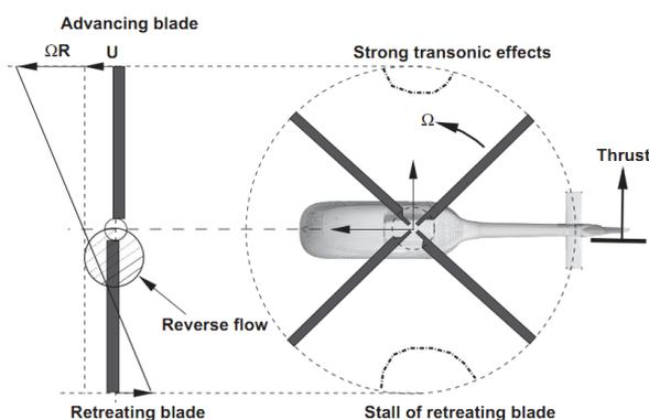
**Fig. 14: Sketch of local speeds on the blade during forward flight and dissymmetric effects [18, p. 338]**
