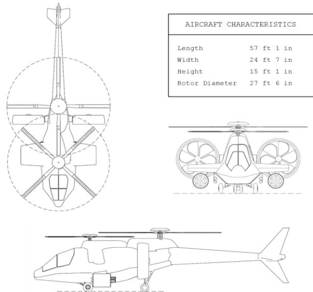
**Fig. 3: Technical aspects of Pankl Aerospace's rotary-wing aircraft concept "H.E.R.O." [2]**
