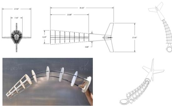
**Fig. 7: 3D and physical model of a bendable tail for the H.E.R.O. concept (preliminary version)**
