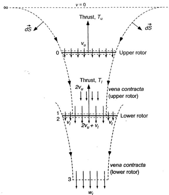
Fig. 11: Hover condition for a coaxial system with stream tube around the two rotor disks [19, p. 102]
