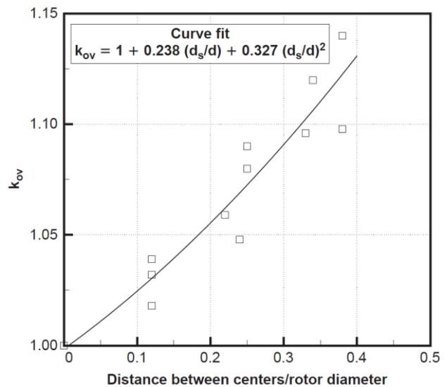
**Fig. 13: Overlap factor for tandem rotors [18, p. 374]**
