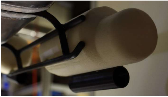
Figure 1: Drawing of the helicopter model including the model-fixed coordinate system (a), and close-up view of one front float equipped with a scoop (b)
