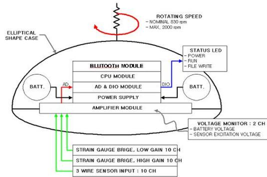
Fig. 26. The DAQ system on the rotating rotor
