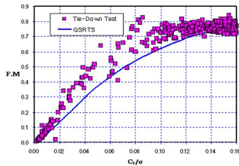
Fig. 22. Figure of merit Comparison of hover test on GSRTS and tie-down test of KURS helicopter
