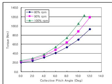
(b) Torque v.s. Collective pitch angle
