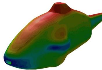
Fig. 15 The Cp contour of new fuselage cover
