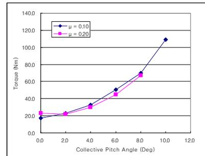
(b) Torque v.s. Collective pitch angle
