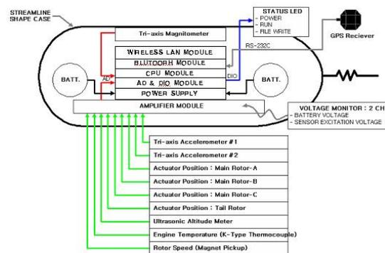
Fig. 27. The DAQ system under the fuselage
