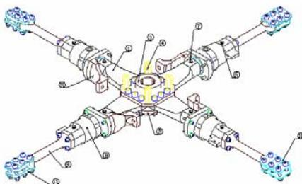
Fig. 9. KURS hub for ground test
