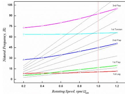
Fig. 13. Calculated frequency distribution for KURS rotor system.
