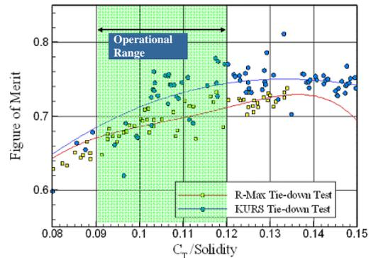
Fig. 23. Figure of merit comparison of the R-Max and KURS based on tie-down test.
