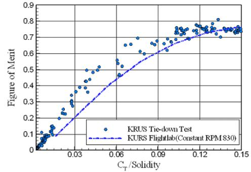
Fig. 21. Comparison of analysis and tie-down test result for KURS helicopter
