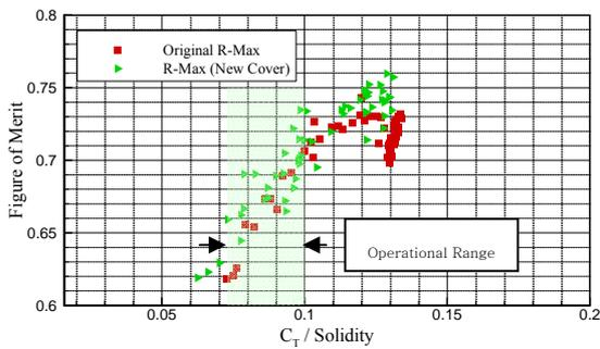
Fig. 29. Figure of merit comparison of original R-Max and R-Max with a new cover
