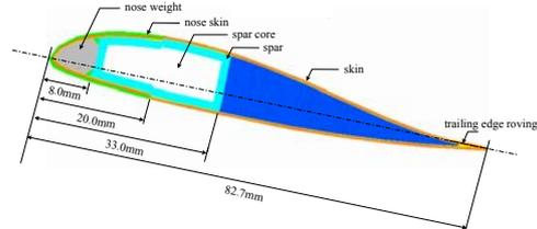
Fig. 10. The typical section of KURS Blade
