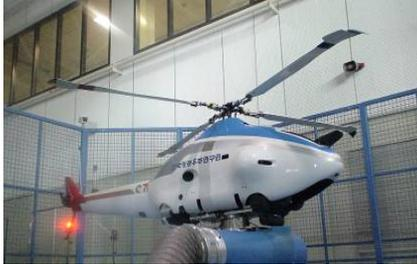
Fig. 20. KURS helicopter installed on the Tie-down test rig
