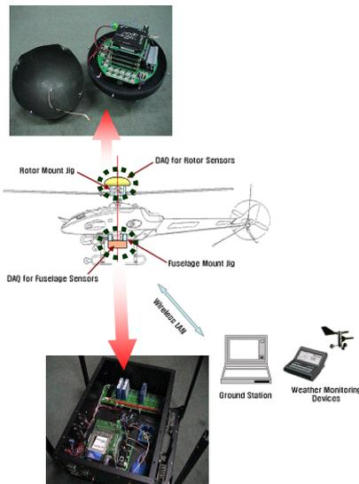
Fig. 25. The general DAQ system on the Flight Test Model
