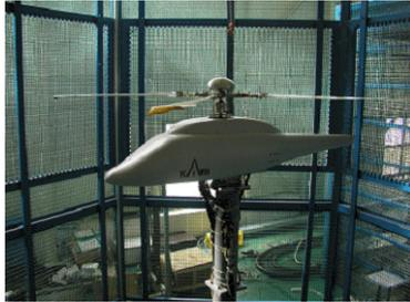
Fig. 16. Hover test installed on KARI GSRTS
