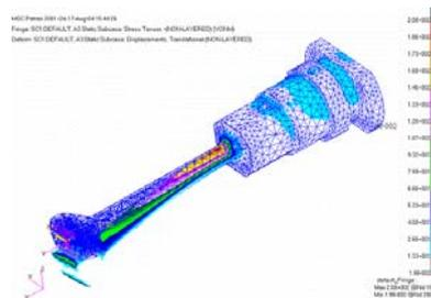
Fig. 11. Nastran analysis result at hover condition
