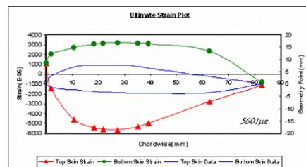
Fig. 12. typical strain results based on Euler beam theory
