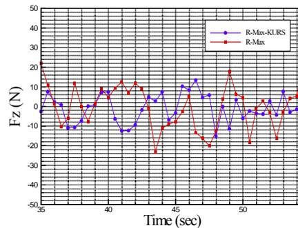
Fig. 33. Vibratory Load ( $F_z$ ) of KURS vs. R-Max
