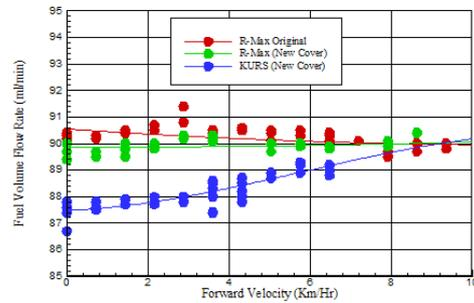
Fig. 32. Comparison of fuel flow rate among R-Max and KURS helicopter.
