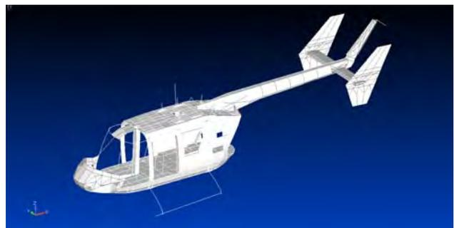
Figure 23: Finite Element airframe model of BK117
