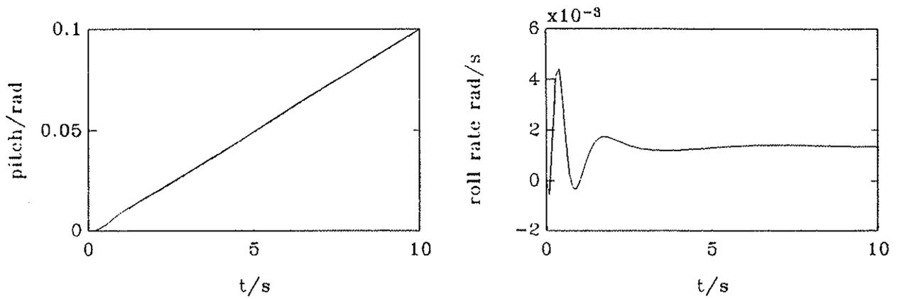
Fig 4: Pitch attitude and roll rate response to a step input on the second inceptor.
