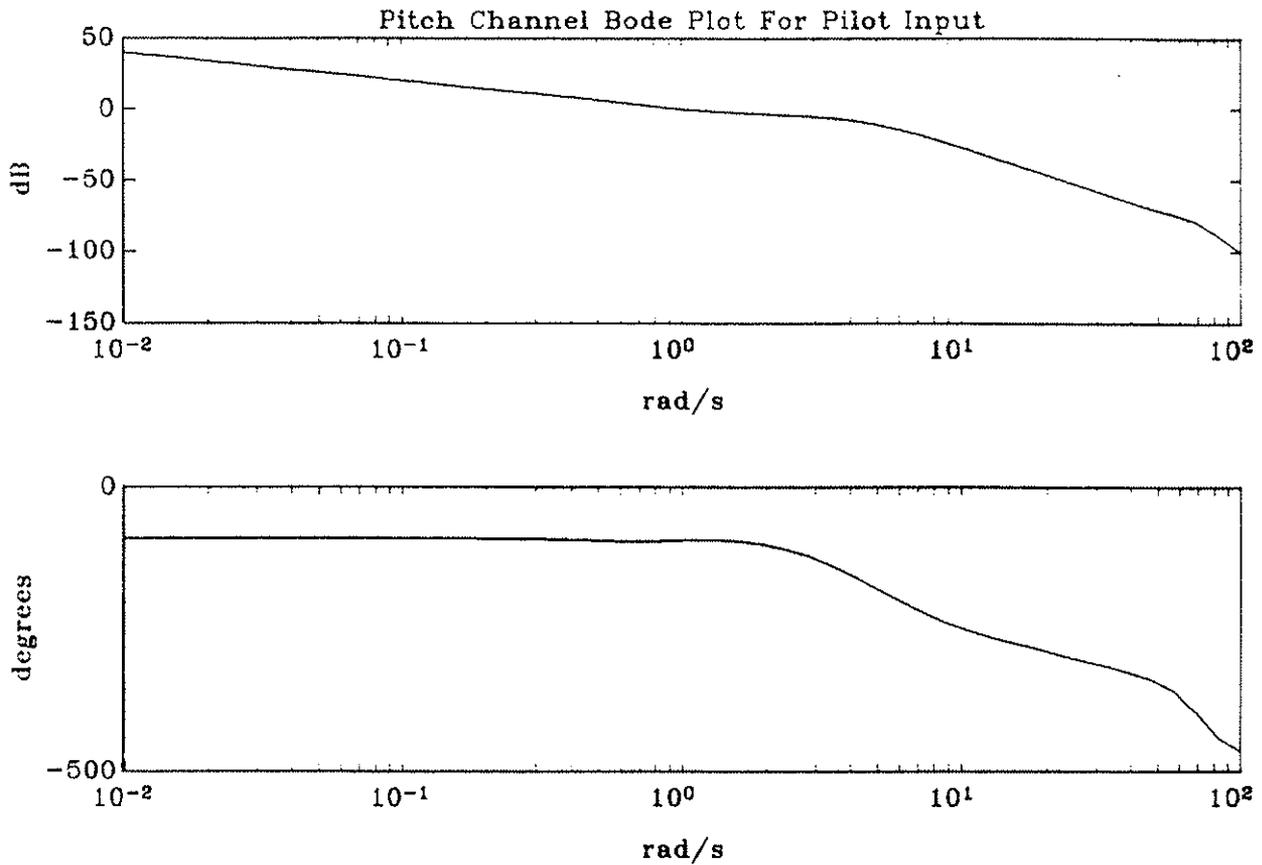
Fig 5: Bode plot for frequency response of pitch attitude from second inceptor.
