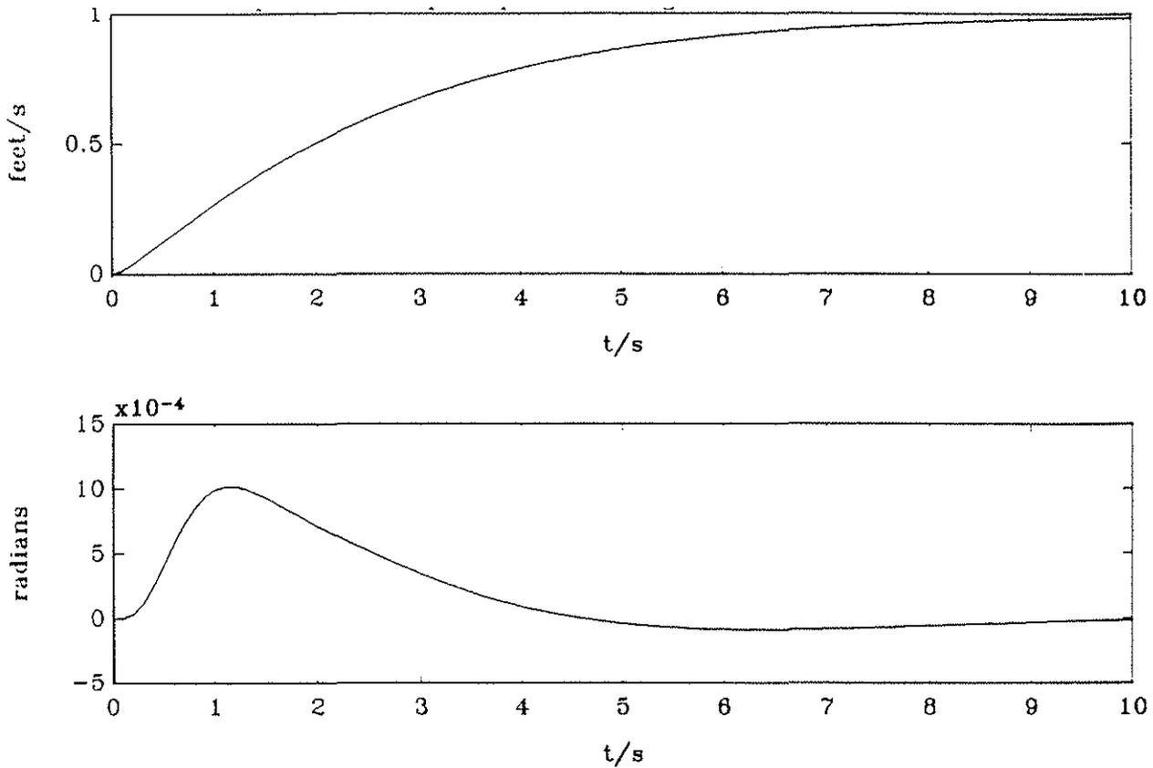
Fig 3: Height rate and pitch attitude response to unit step on first inceptor.
