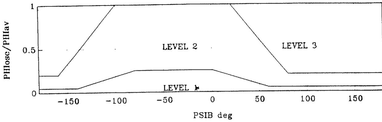
Fig 6: Handling qualities plot for bank angle oscillations requirement.
