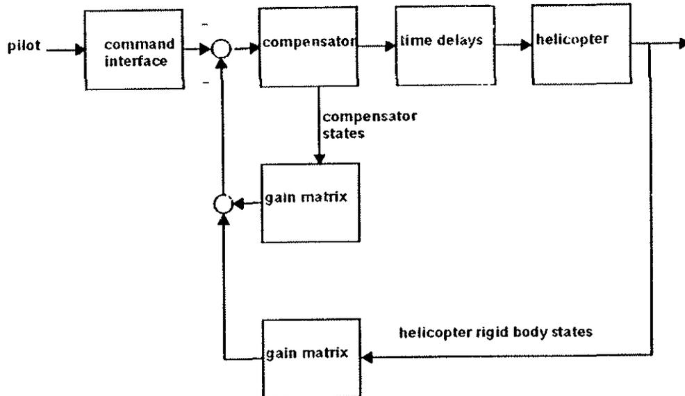
Fig 1: Control design block diagram including time delays used at design stage.
