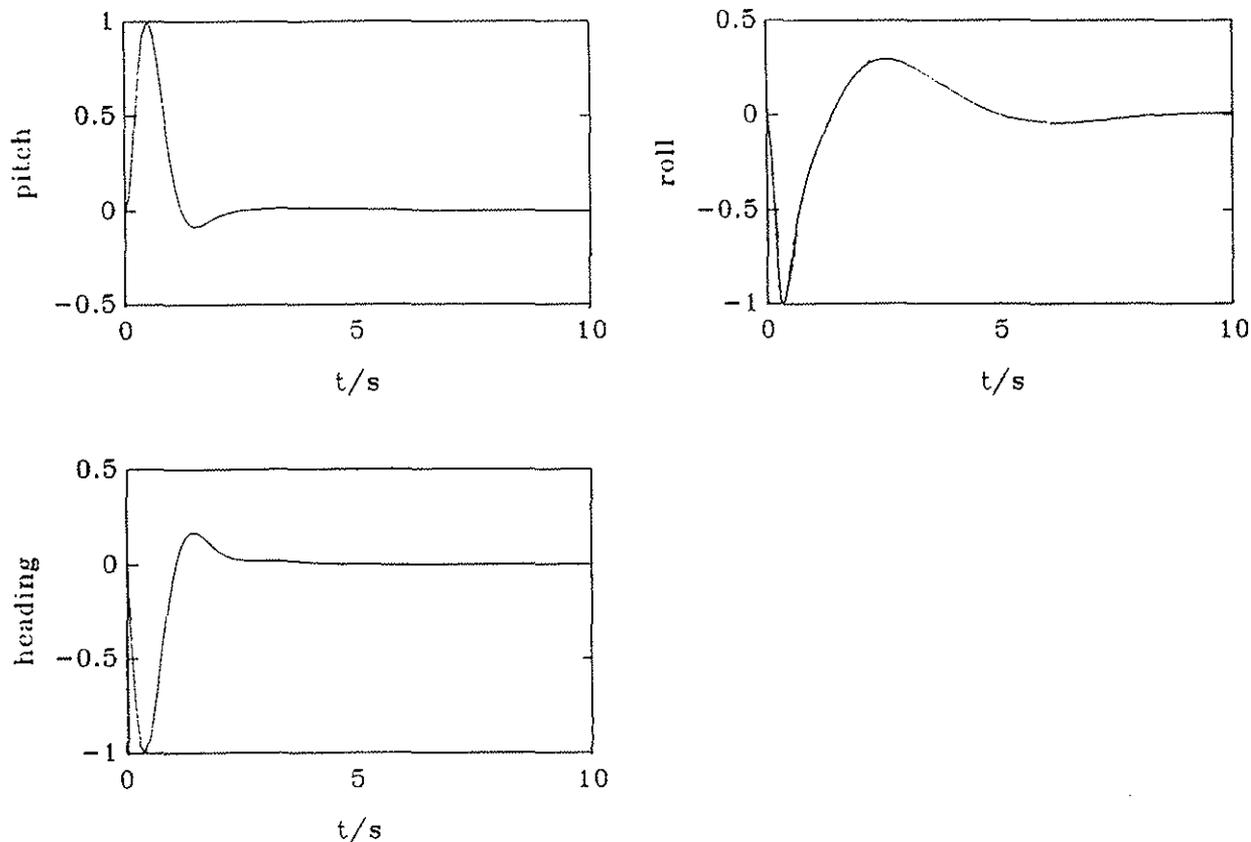
Fig 2: Simulated attitude and heading responses to impulses input directly to actuators. (Normalised so peak excursion is one).
