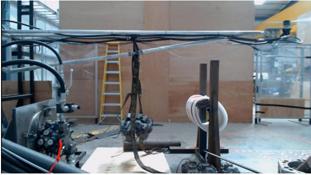
Figure 9 : Phase Two test rig lifting 85kg; the pump is in the foreground on the left.
