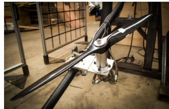
Figure 8 (top) Phase one single axis test rig and time domain response result (bottom) detail of motor and prop
