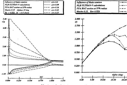
Fig.9: Calculated pressure distributions for rotating blade, geometry of fig.8.
