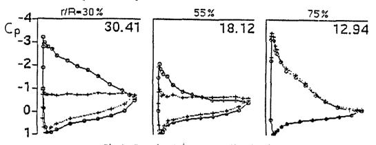
Fig.8: Experimental pressure distributions for the rotating blade (circle) and the non-rotating blade (cross).
