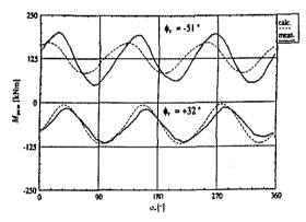
Fig.4: Contribution of blade bending moments to restoring yaw moment at 32° and -51° yaw angle. Comparison of measurements and calculations. Definition azimuth angle: see fig.5.
