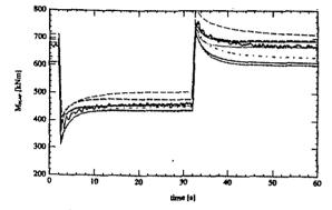
Fig.1: Measured and predicted flapping moments at blade root. Measured data: irregular full line.
