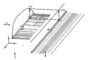
Fig.3: Definition of induced velocity at P; sum of contributions of vortex systems A and 8.
