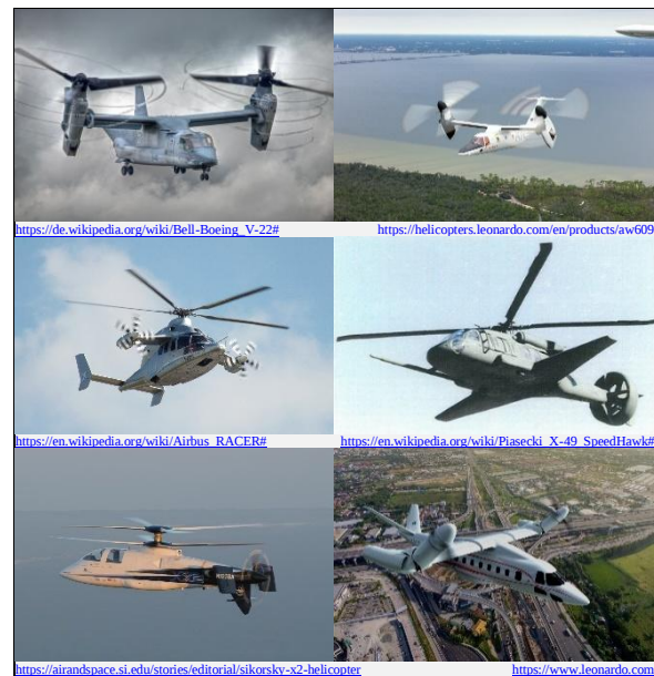
Figure 1: Convertiplane and Compound Helicopters
