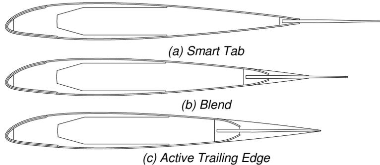
Figure 2: Smart tab versus Active Trailing Edge
