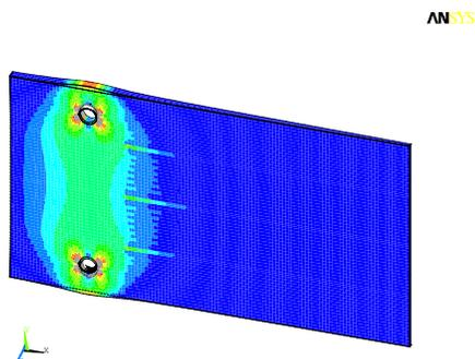
Figure 11: ANSYS model of the bending actuator:
