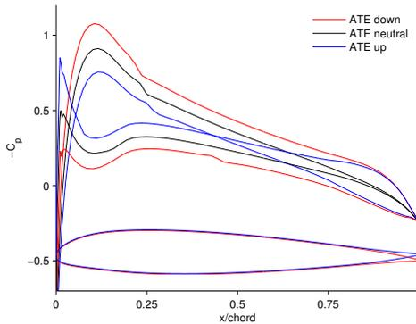
Figure 7:  $C_p(x)$  for deflected airfoil at  $\alpha = 0^\circ$  and  $Ma = 0.6$  calculated with XFOIL
