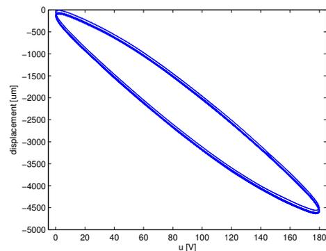
Figure 10: active deflection of a ATE bender module at full operating voltage
