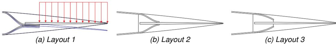
Figure 8: Connection of Active Trailing Edge and passive blade structure
