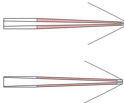
Figure 5: Optimized thickness distribution of active and core layers for different constraints
