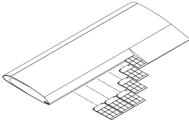
Figure 9: Integration of actuator modules into rotor blade segment
