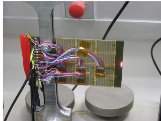
Figure 12: Active Trailing Edge bending actuator
