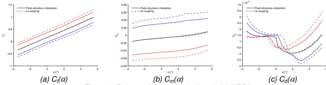
Figure 6: Polars at  $Ma = 0.6$  calculated with XFOIL
