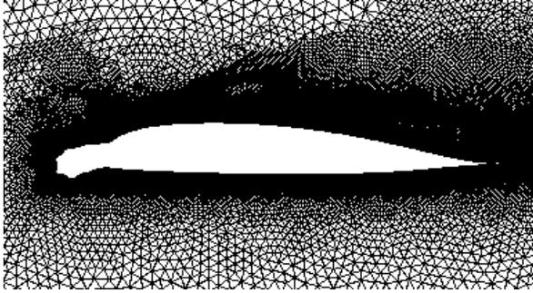
Figure 16: Unstructured grid around ice shape 2
