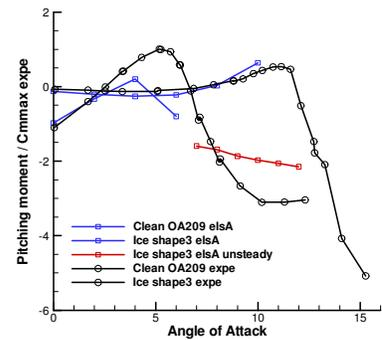
Figure 31: Pitching moment coefficient for the clean and iced OA209 at Mach 0.5
