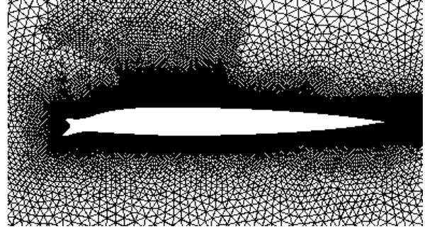
Figure 17: Unstructured grid around ice shape 3
