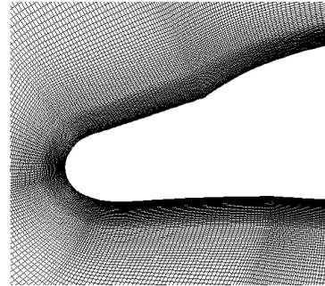
Figure 9: Structured grid around ice shape 1
