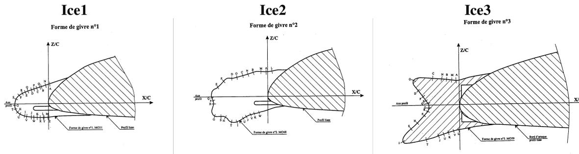
Figure 3: Iced-leading edges used for wind tunnel tests
