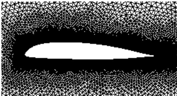
Figure 14: Initial unstructured grid around clean OA213
