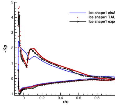
Figure 34: Pressure coefficient distribution on the ice shape1 at Mach 0,3 and  $10^\circ$  angle of attack
