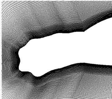
Figure 10: Structured grid around ice shape 2
