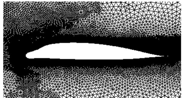
Figure 15: Unstructured grid around ice shape 1
