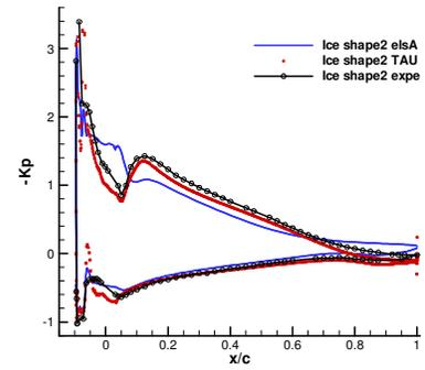
Figure 35: Pressure coefficient distribution on the ice shape2 at Mach 0,3 and  $8^\circ$  angle of attack
