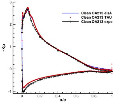
Figure 33: Pressure coefficient distribution on the clean and iced OA213 at Mach 0,3 and  $10^\circ$  angle of attack
