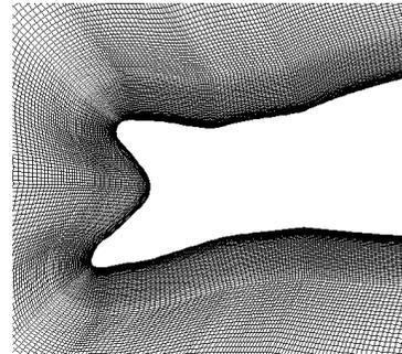
Figure 11: Structured grid around ice shape 3
