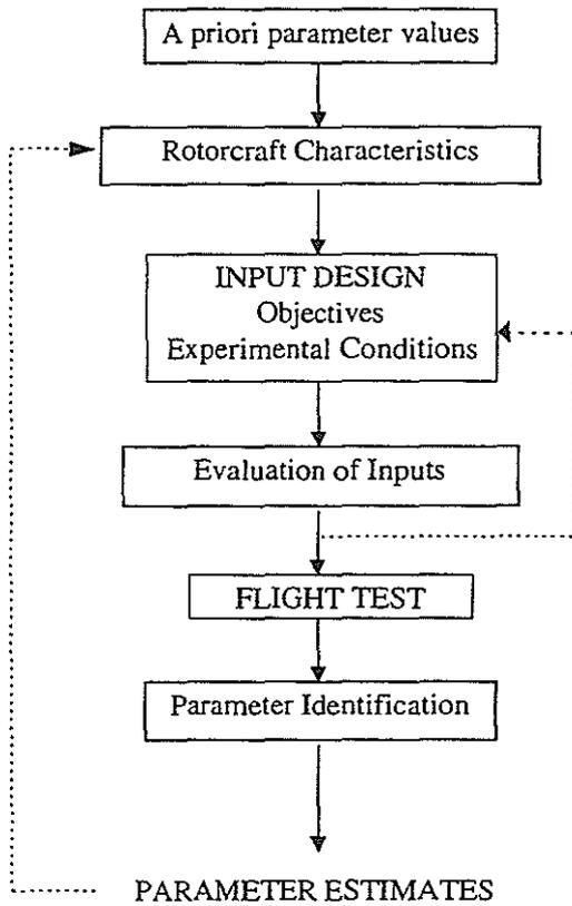
Fig 2 : Identification Procedure
