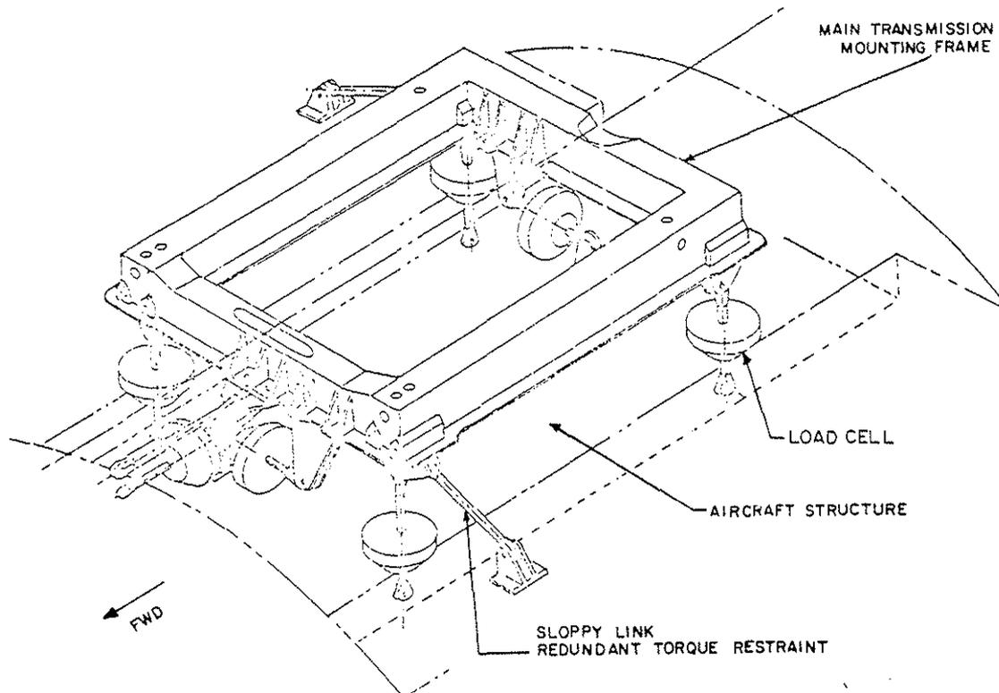
Figure 5. Baseline RSRA Load Cell Transmission Support System.
