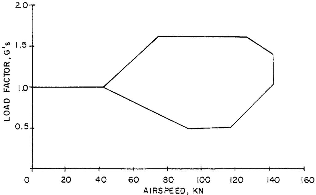
Figure 17. RSRA Load Factor/Airspeed Envelope with Active Isolator, Helicopter Configuration.
