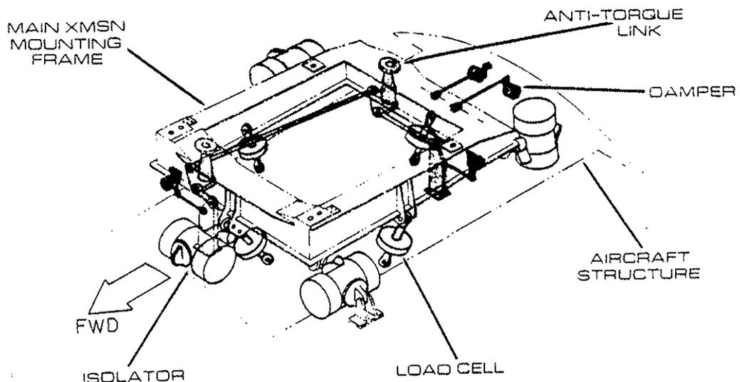
Figure 4. RSRA Transmission Active Isolation Rotor Balance System.
