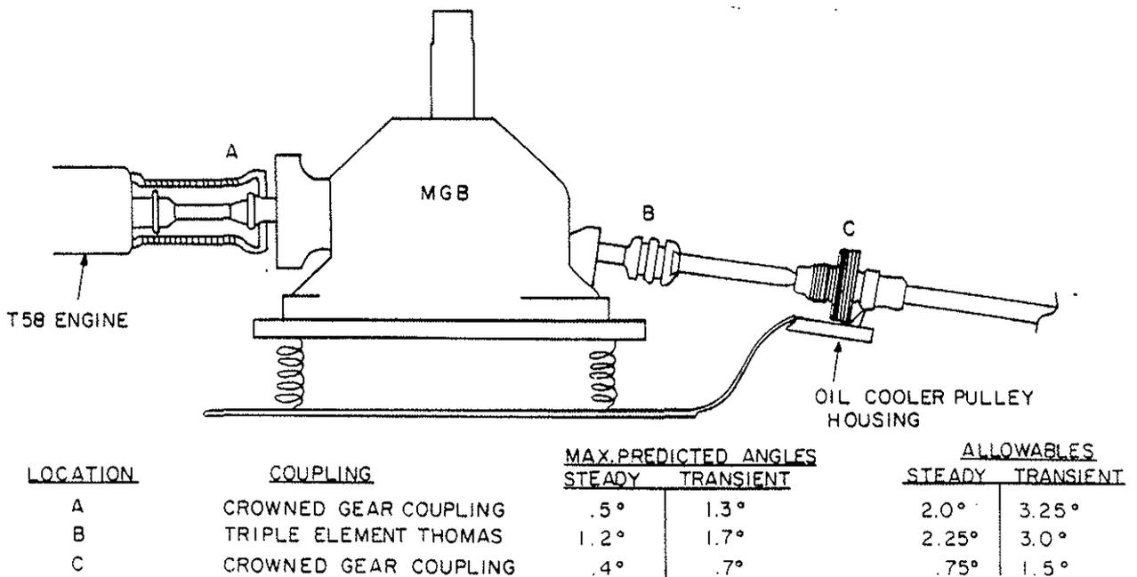
Figure 11. RSRA Transmission/Airframe Misalignments.
