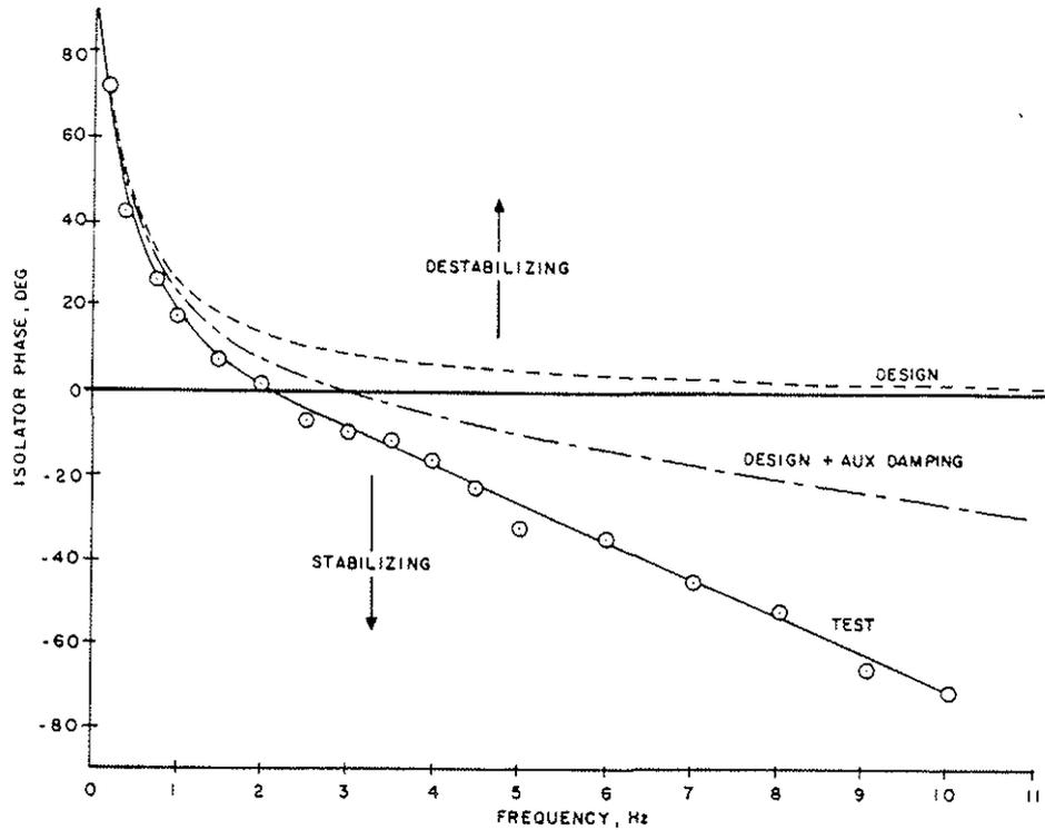
Figure 13. Lateral Isolator Phase Response Characteristics.
