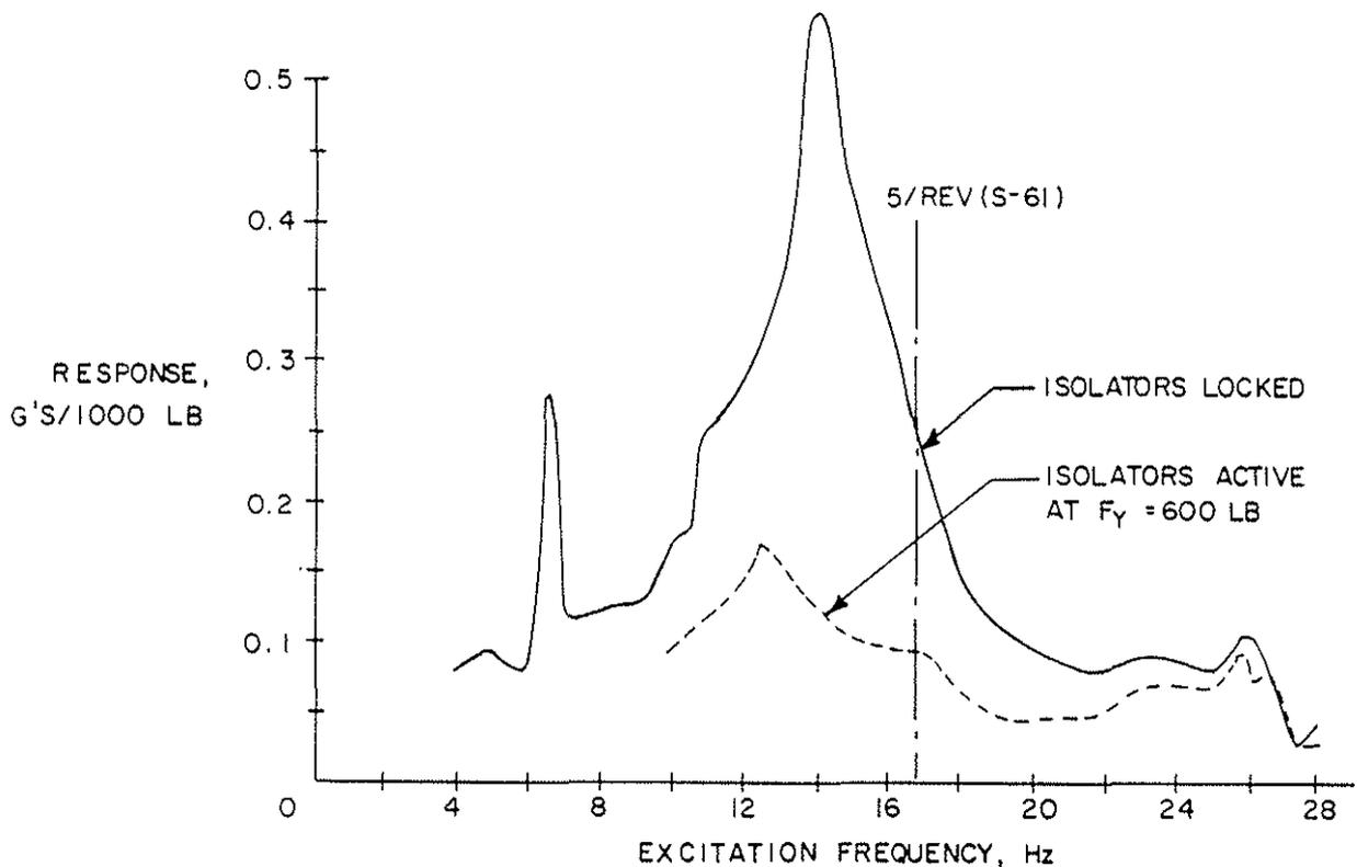
Figure 16. Evaluation Pilot Vertical Response to MRH Lateral Excitation Force (RSRA Shake Test).
