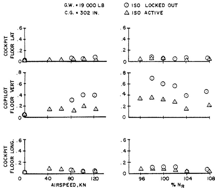
Figure 21. RSRA Vibration with Active Isolator.
