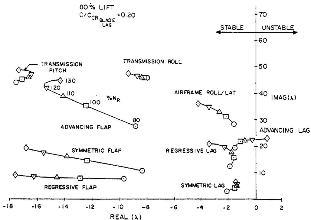
Figure 6. RSRA/AIBS Ground Resonance Stability.
