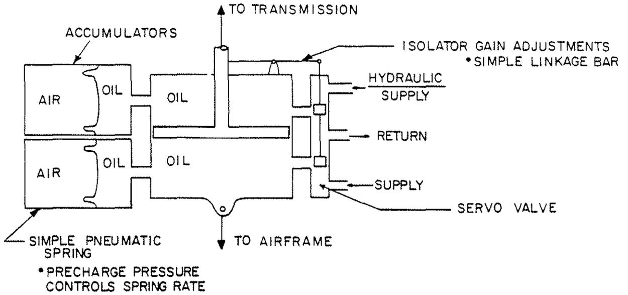
Figure 2. Schematic of Hydropneumatic Active Isolator.
