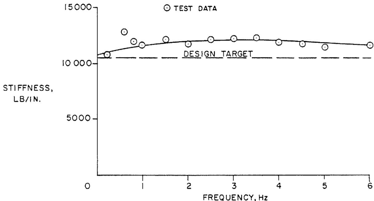
Figure 12. Lateral Isolator Effective Stiffness From Performance Test Results.
