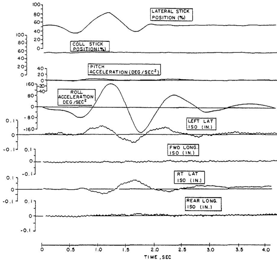
Figure 20. Illustration of Isolator Active Centering Feature During Maneuvering Flight.
