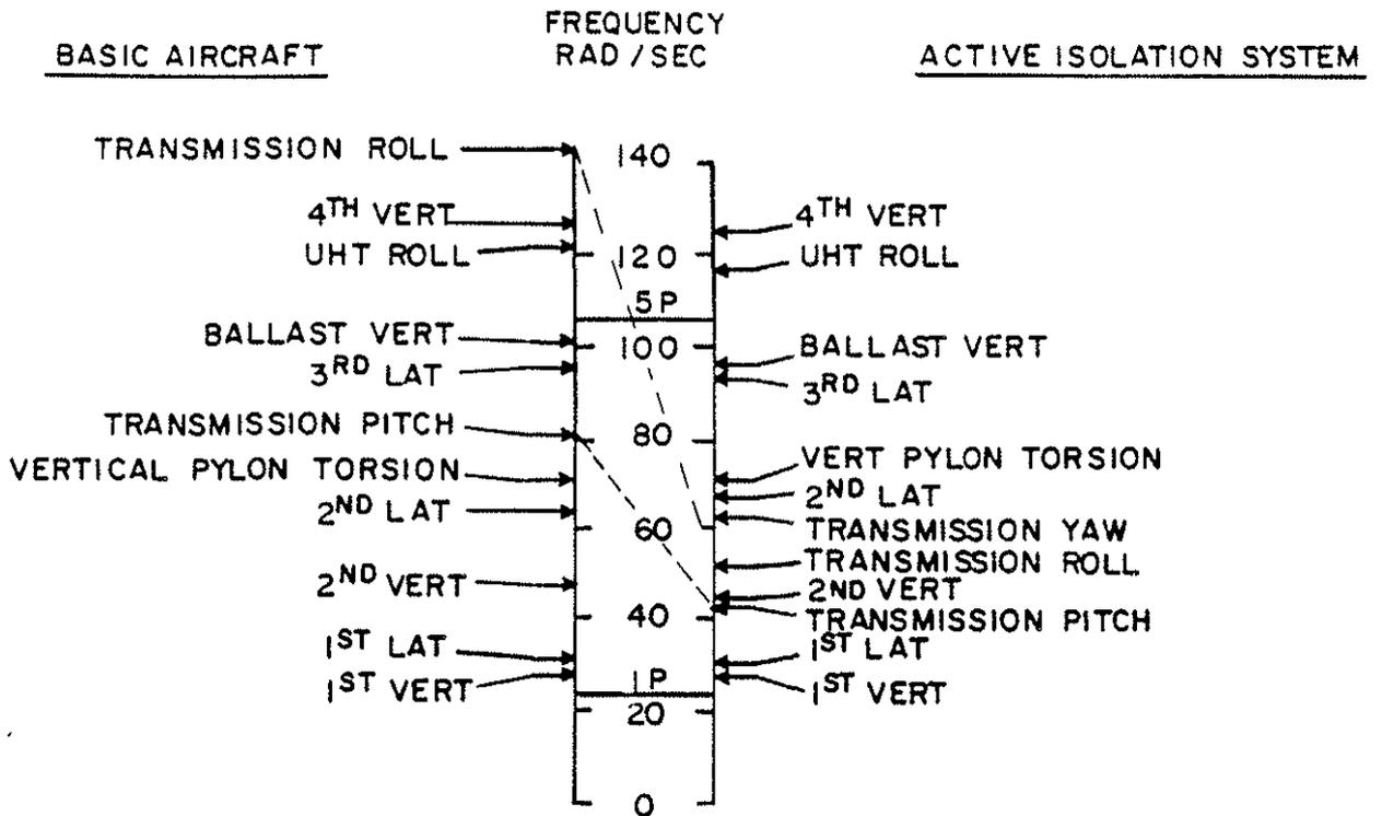
Figure 10. Effect of Active Isolator on RSRA Helicopter Airframe Mode Frequencies.
