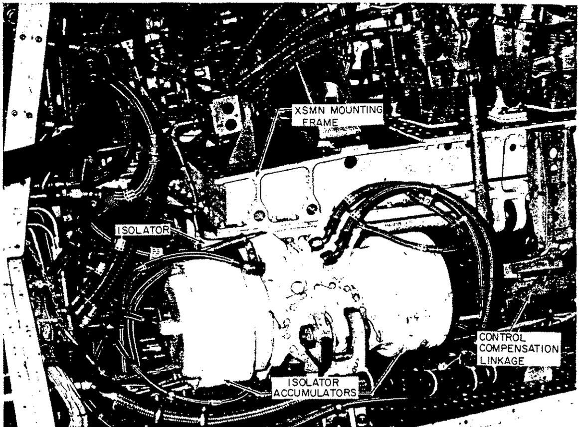
Figure 3. Right Rear Lateral Active Isolator Installed in RSRA.
