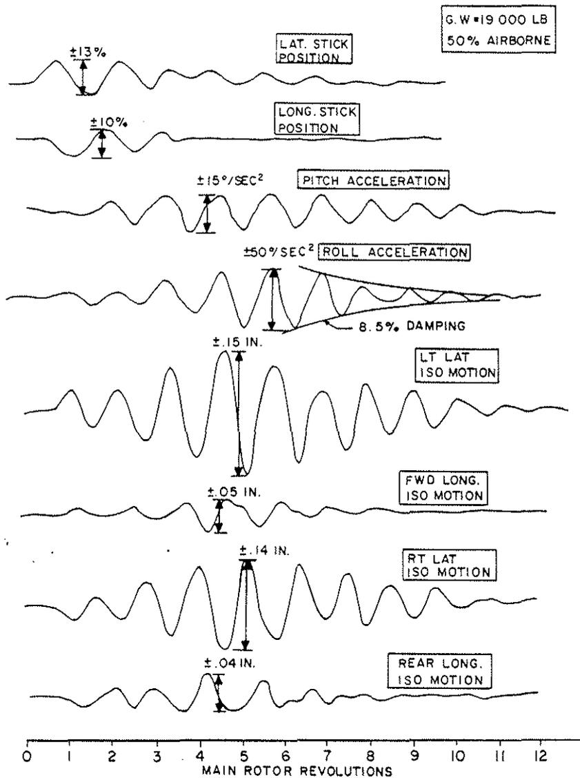
Figure 18. RSRA/AIBS Mechanical Stability Test Data.
