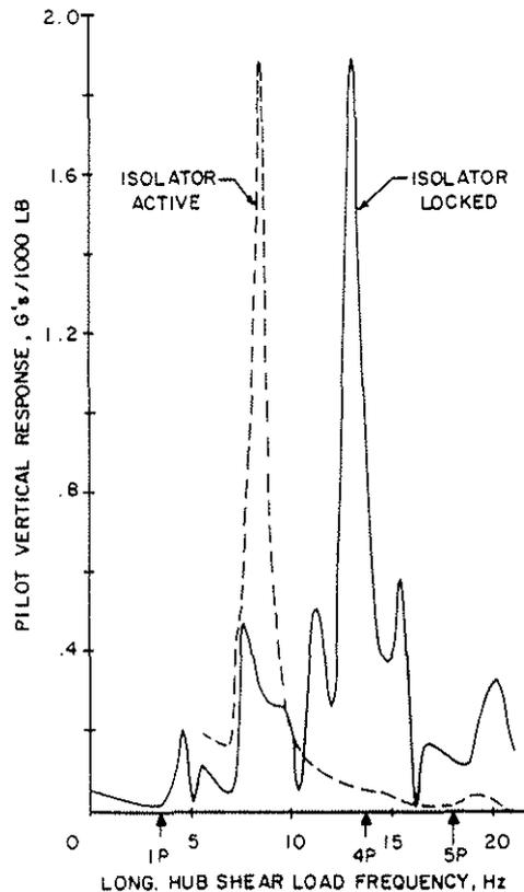
Figure 9. Predicted Transmission Mode Detuning by Active Isolator.
