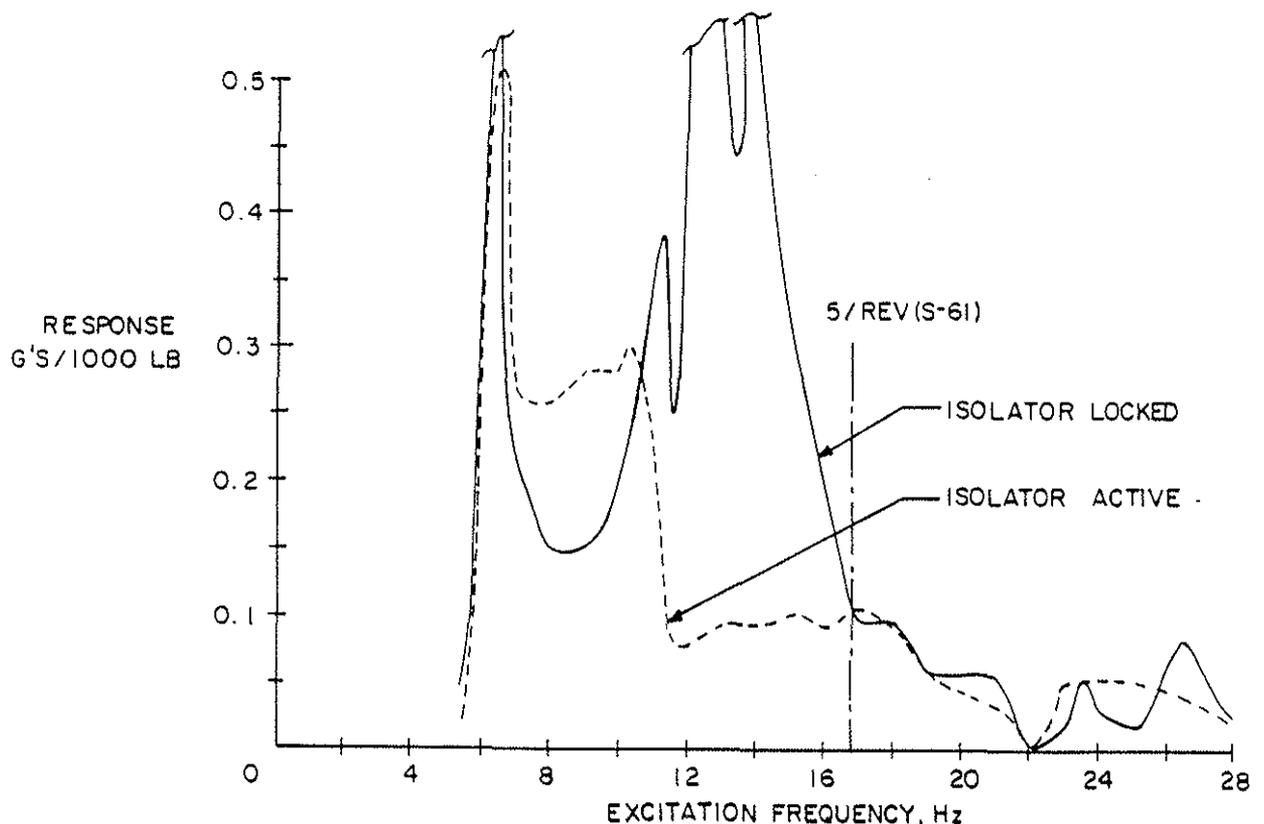
Figure 15. Pilot Vertical Response to MRH Longitudinal Excitation Force (RSRA Airframe Shake Test).
