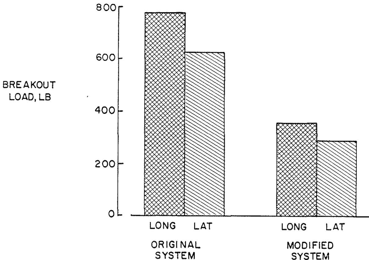
Figure 14. System Static Breakout Loads @ V = 120 kts
