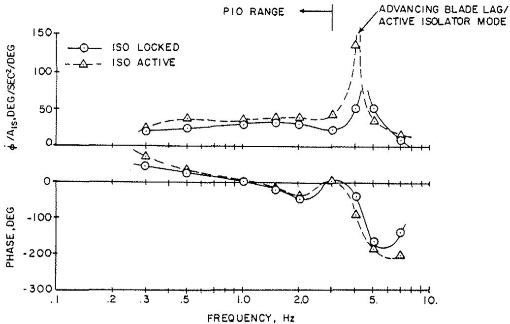
Figure 8. Effect of Active Isolator on RSRA Handling Qualities .
