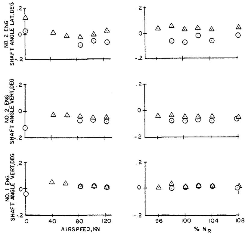
Figure 19. Engine Shaft Misalignments with Isolation System Active.
