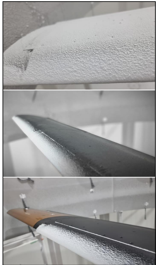
Figure 19: Different icing configurations during the first icing with the deicing blade, A: de-icing blade, A: de-icing blade , A: de-icing blade and reference
