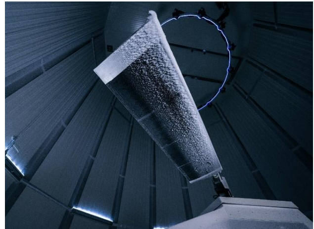
Figure 16: First icing tests in whirl tower, lower side of the test body
