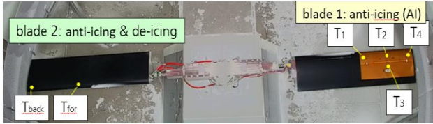
Figure 18: De-icing test in the whirl tower, de-icing blade (left) and reference blade (right)
