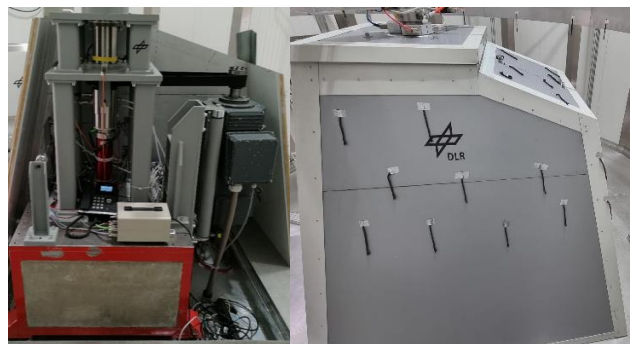
Figure 6: Enclosure of rotor test rig, left: open, right: closed
