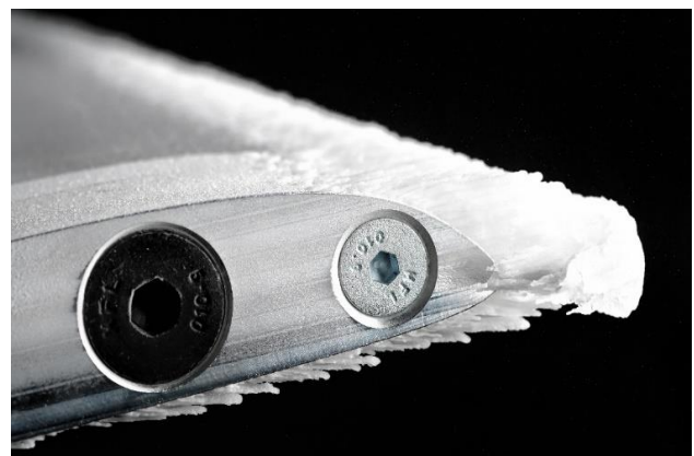
Figure 17: Accumulation of ice at the leading edge of the test specimen
