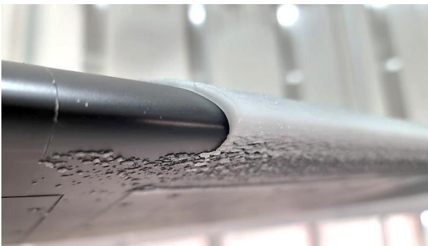
Figure 23: Chipped ice on the leading edge of the test rotorblade
