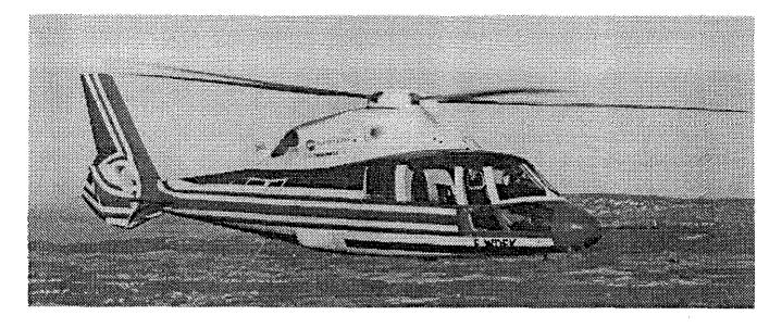
Flight controls: A Dauphin helicopter has now been flown with Fly-By-Wire controls, a conventional stick to begin with and now a mini-stick. It is thought that this technique is now mastered well enough to be on offer in NH90. Most of the work now involves assessing new piloting laws (piloting by objective).
