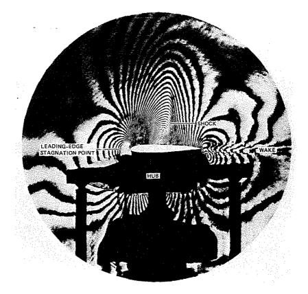
Fig. 17. Interferogram recorded at  $180^{\circ}$  (chordwise view).
