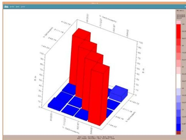
Figure 11: MAC matrix between EMA and OMA - Flight excitation
