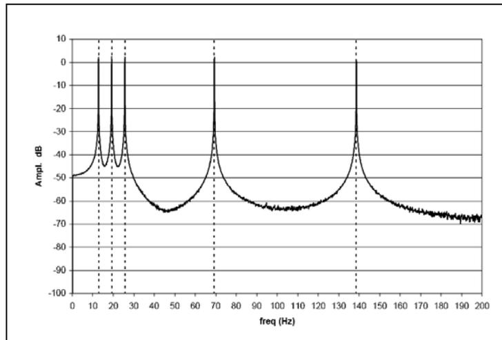
Figure 8: Load spectrum - Tonal excitation
