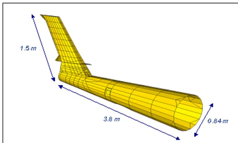
Figure 1: Geometry of the tail
