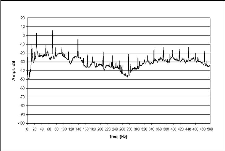
Figure 10: Load spectrum - Flight excitation
