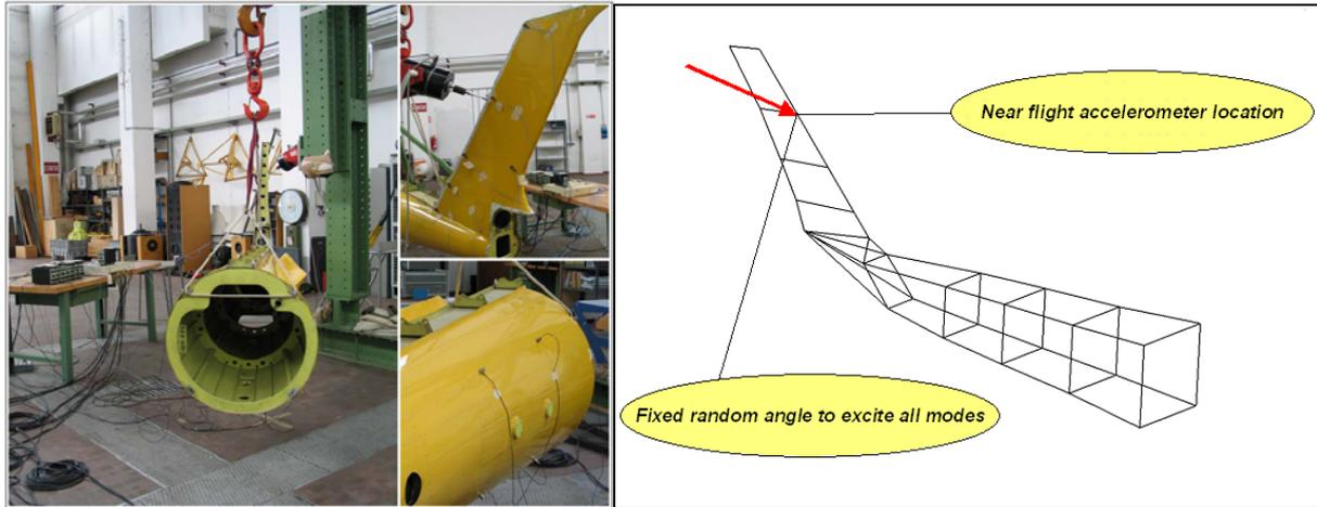
Figure 6: Load application in OMA procedure
