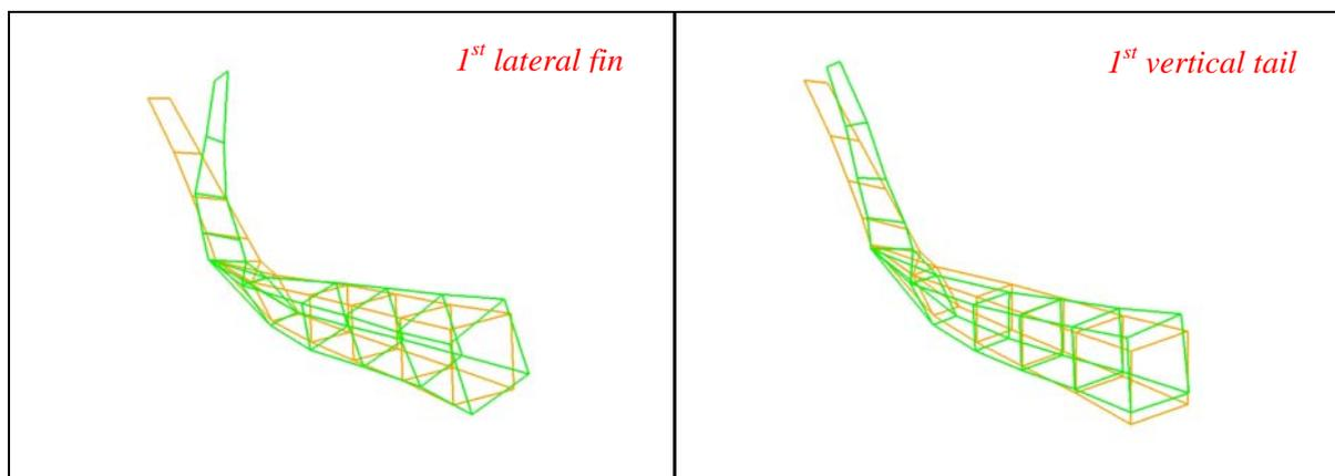
Figure 5: First two modes extracted in EMA procedure
