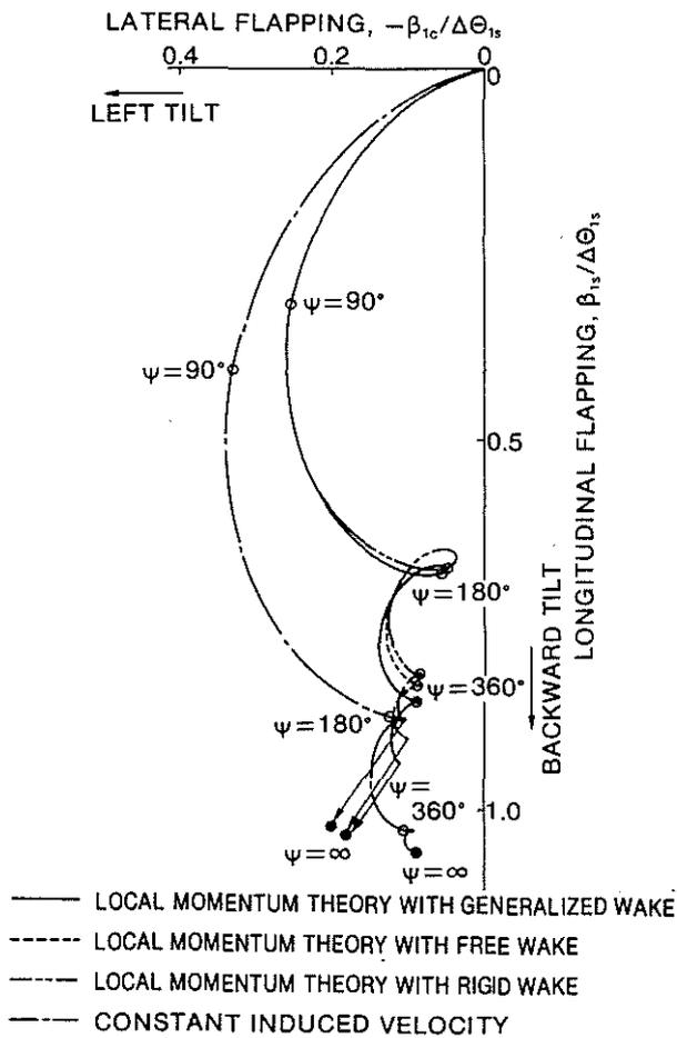
Fig. 8. Inclination of tip path plane caused by a rapid increase of cyclic pitch.
