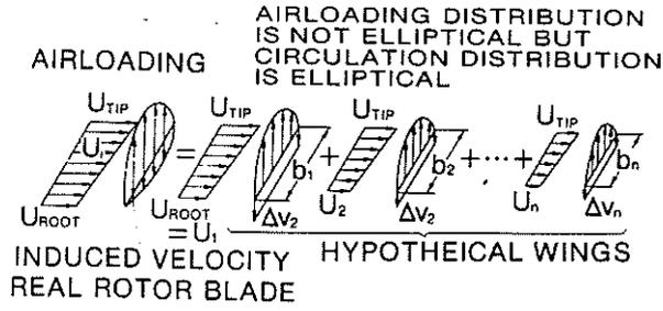
Fig. 2. Decomposition of a rotor blade to hypothetical wings.<sup>7)</sup>
