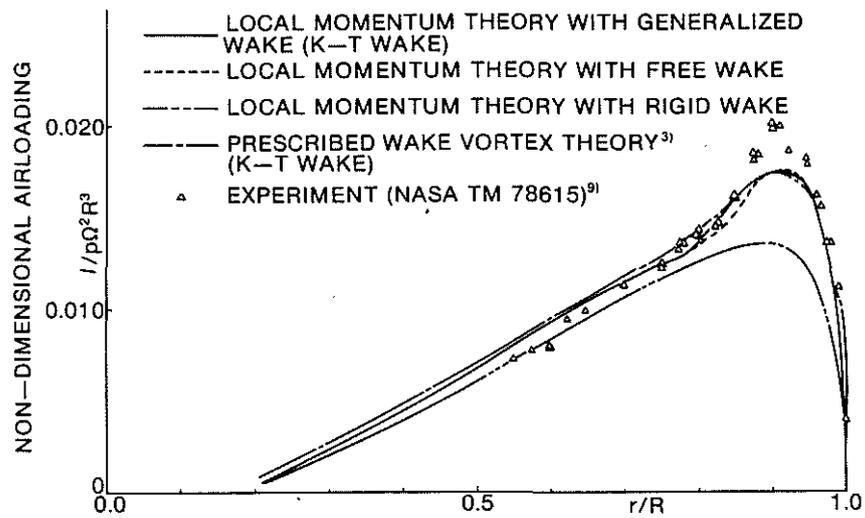
Fig. 5. Span-wise lift distribution in steady state, with Kocurek and Tangler wake model ( $b=2$ ,  $\theta_t=-10.9$  deg.,  $AR=13.7$ ,  $\theta_{0.75}=9.8$  deg.)
