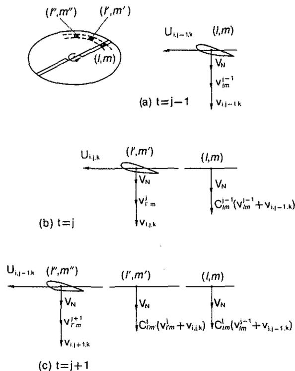
Fig. 1. Time-wise variation of induced velocity on rotor rotational plane.<sup>8)</sup>
