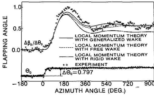
Fig. 7. Transient response of flapping angle caused by a rapid increase of collective pitch.
