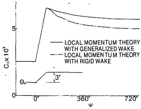
Fig. 6. Transient response of thrust coefficient caused by a rapid increase of collective pitch.
