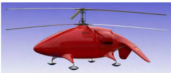
Fig. 1: SHARC coaxial helicopter UAV [EADS].
