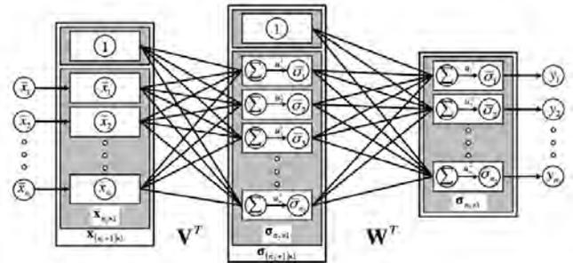
**Fig. 8: Neural Network with input, hidden and output layer and relevant weighting matrices  $V^T$  and  $W^T$  [10].**
