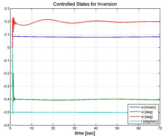
**Fig. 12: Step inputs to controlled system with stabilising proportional controller and adapting online Neural Network in presence of model deviation.**
