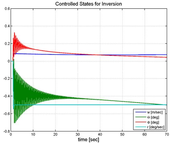
**Fig. 11: Step inputs to controlled system with stabilizing proportional controller in presence of model deviation.**
