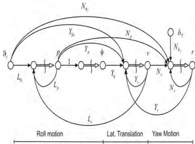
**Fig. 7: Signal flow diagram for Lateral Motion as used in linear Dynamic Inversion.**
