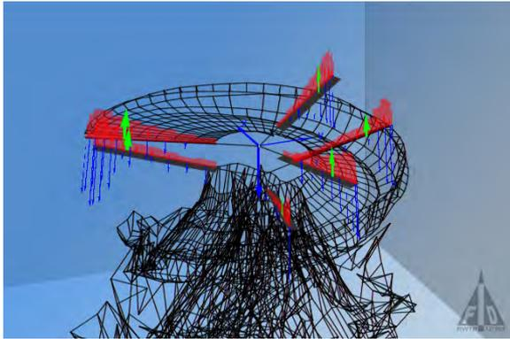
**Fig. 3: Coaxial rotor with wake (shown only for one upper blade) in hover flight. Circulation in red, blade thrust in green and induced velocities in blue.**
