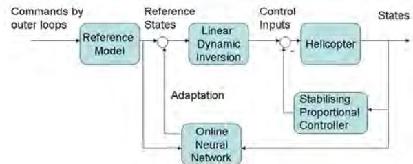
**Fig. 5: Scheme for Basic Controller with stabilizing proportional controller and adaptive Neural Network for Dynamic Inversion.**
