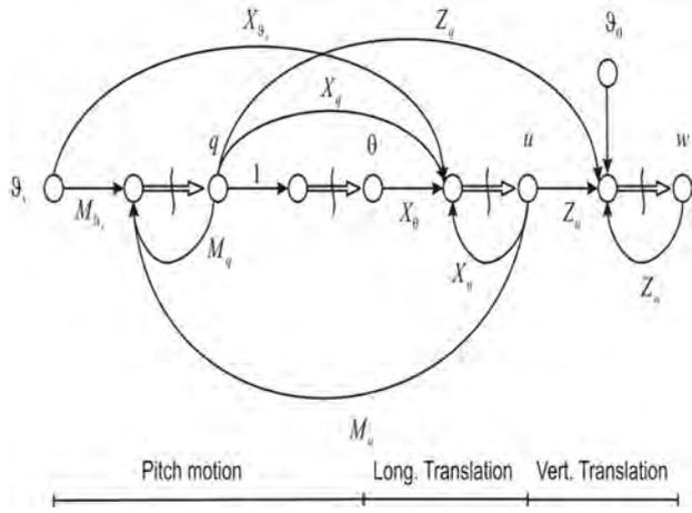
**Fig. 6: Signal flow diagram for Longitudinal Motion as used in linear Dynamic Inversion.**
