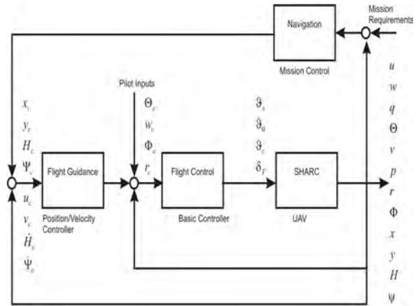
**Fig. 4: Overall structure of the FCGS.**
