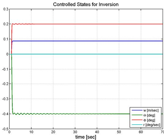
**Fig. 10: Step inputs to controlled system with inversion and stabilizing proportional controller.**
