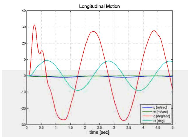
**Fig. 14: Non-linear simulation of longitudinal motion for pitch oscillation with inversion, stabilizing controller and online Neural Network.**
