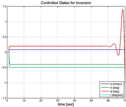
**Fig. 9: Step inputs to controlled system with inversion only and following instability due to numerics.**
