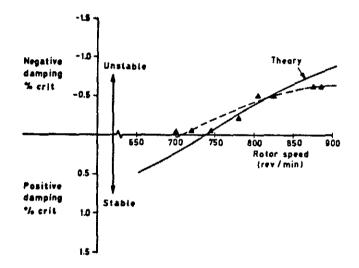
Fig 3 Ground resonance instability at 12<sup>0</sup> collective pitch
