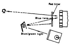
Fig 4 Shared aperture system for viewing instruments
