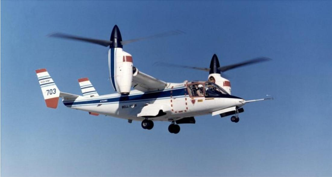
Figure 1 XV-15 in low-level hover mode flight (NASA photo)
