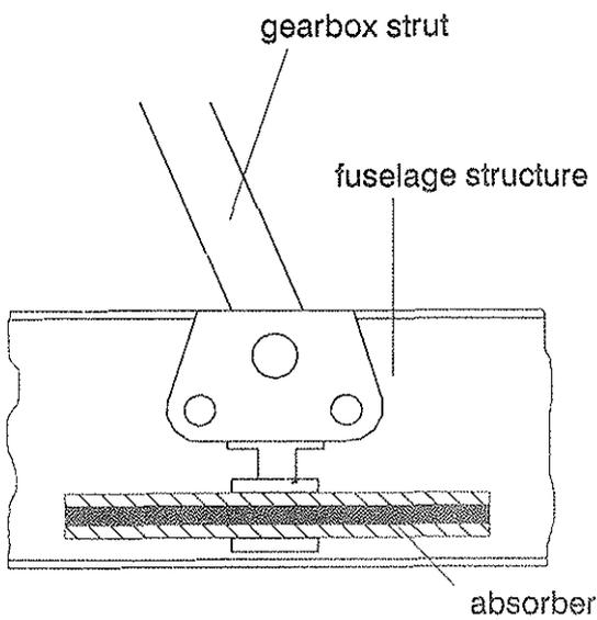
Figure 21: Schematic Diagram of the Test Arrangement Inside the Helicopter
