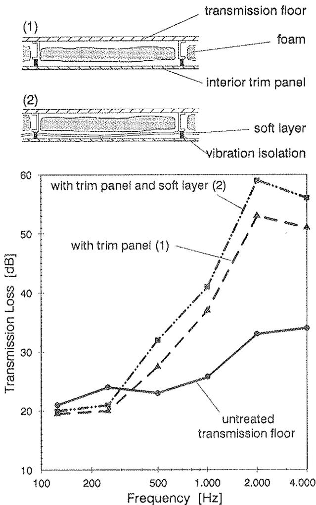
Figure 7: Sound Attenuation of a Transmission Floor
