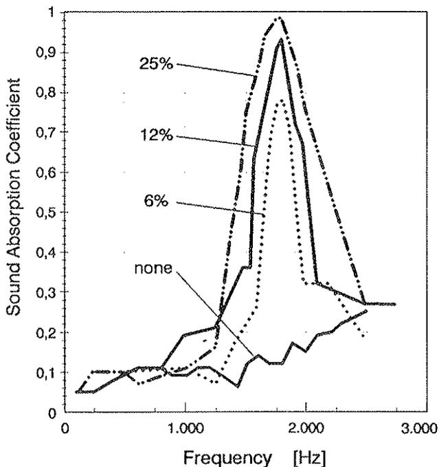
Figure 10: Absorption of the Honeycomb Separation Wall by Different Number of Honeycomb Cores Converted to Resonators (6%, 12%, 25%)
