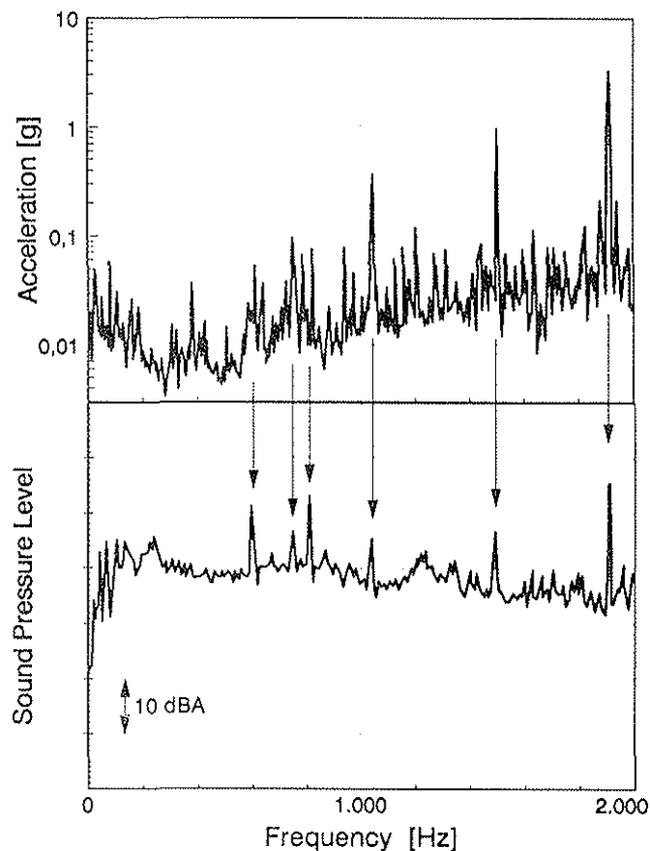
Figure 19: Gearbox Mount (Z1) Acceleration and Cabin Sound Levels of the BK 117
