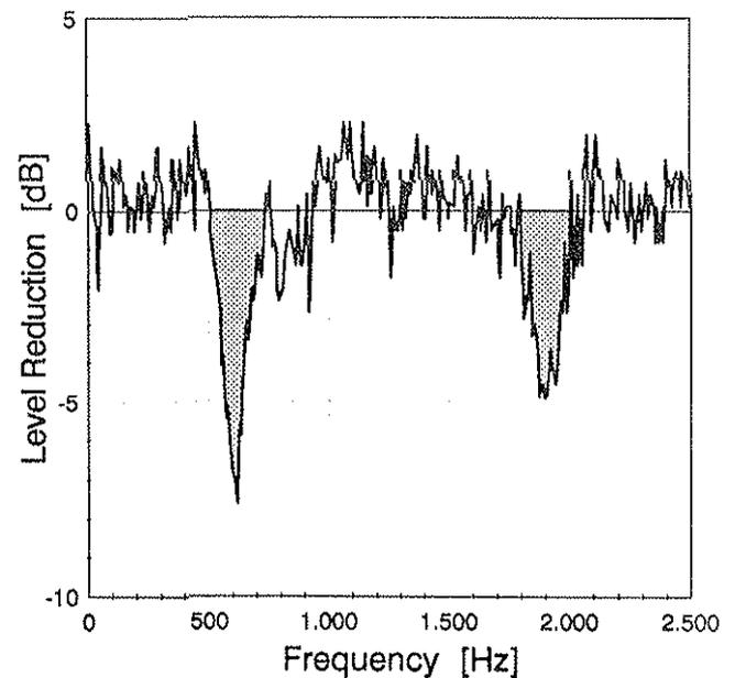
Figure 14: Noise Level Reduction of the Headrest Resonator System in Flight Test
