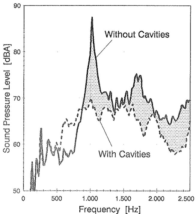
Figure 17: Noise Level Measurements With and Without Resonator Ring
