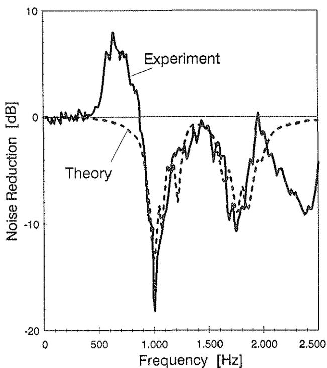
Figure 18: Estimation of the Expected Noise Reduction by the Resonator Ring Compared with Measurement Results
