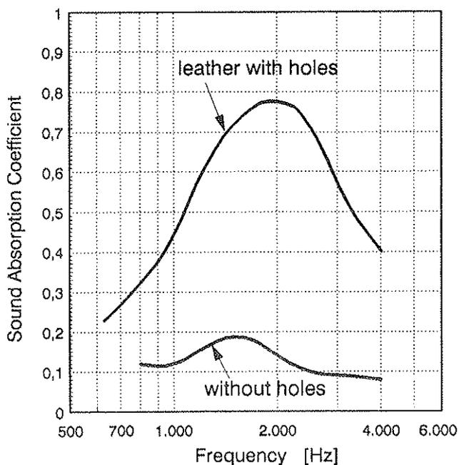
Figure 11: Sound Absorption of a Perforated Leather Cover
