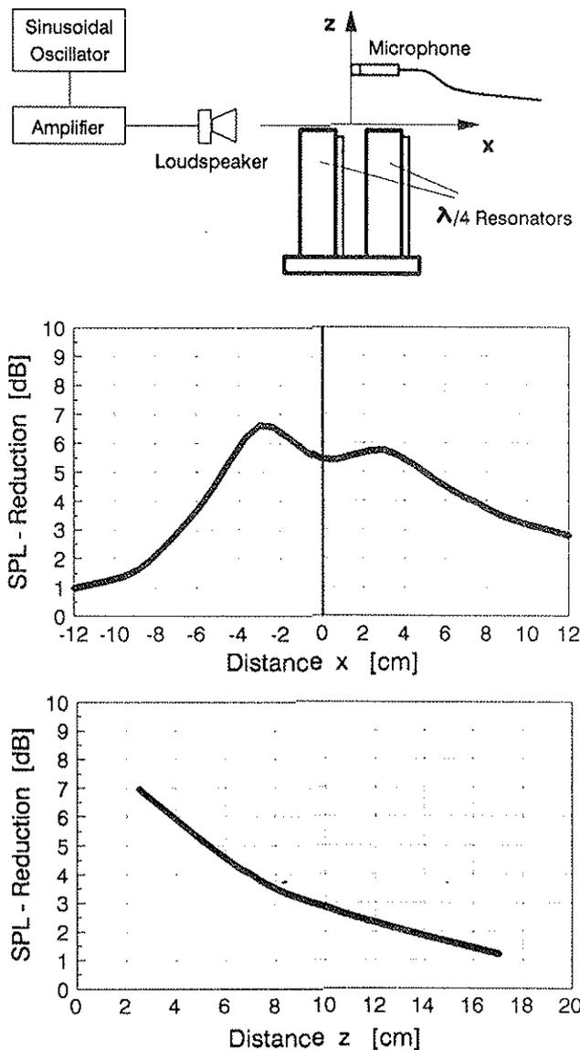
Figure 12: Preliminary Investigation of the Distance Efficiency of Resonators
