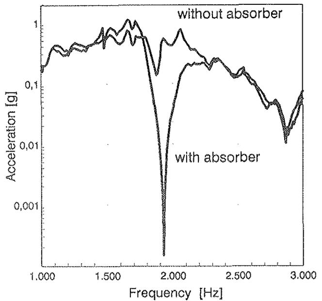
Figure 22: Vibration Transmission Frequency Response of Gearbox Strut Z1 With and Without Absorber
