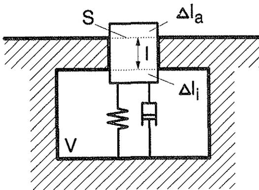
Figure 8: Helmholtz Resonator
