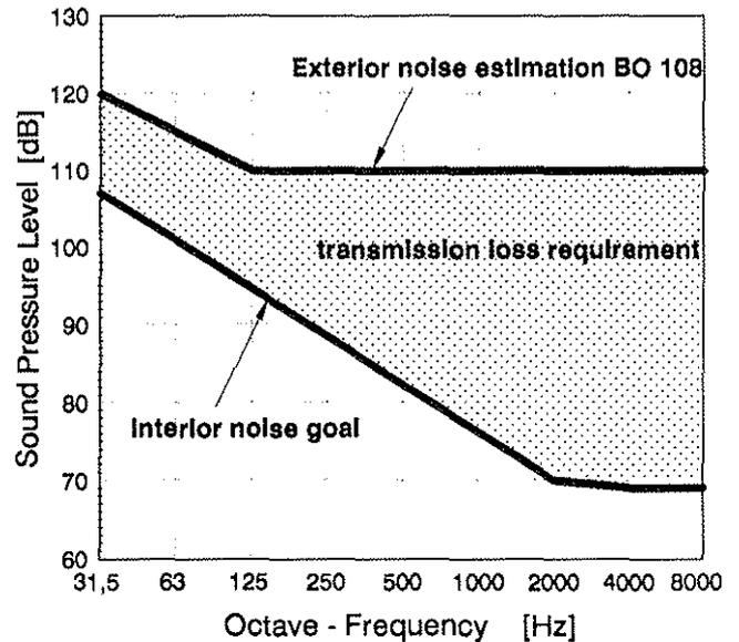
Figure 2: Standard Interior Noise Requirement and Prediction of the External Noise Loading on the BO 108 Cabin Roof
