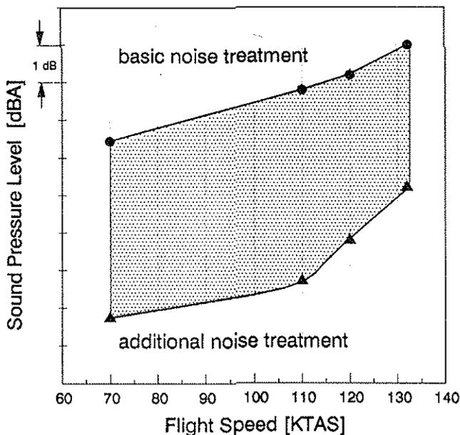
Figure 23: BK 117 Measurement Results Before and After Additional Noise Treatment
