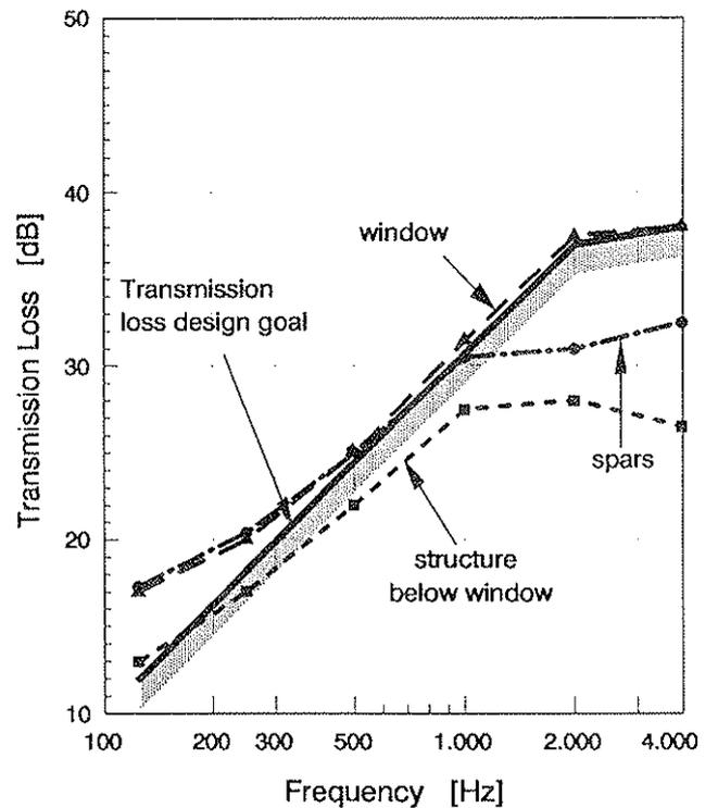
Figure 5: Transmission Loss Measurements of the BO 108 Cabin Door, Basic Design
