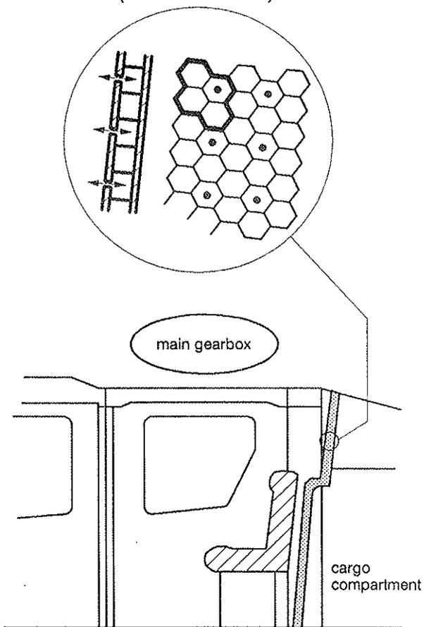
Figure 9: Resonators in a Bulkhead
