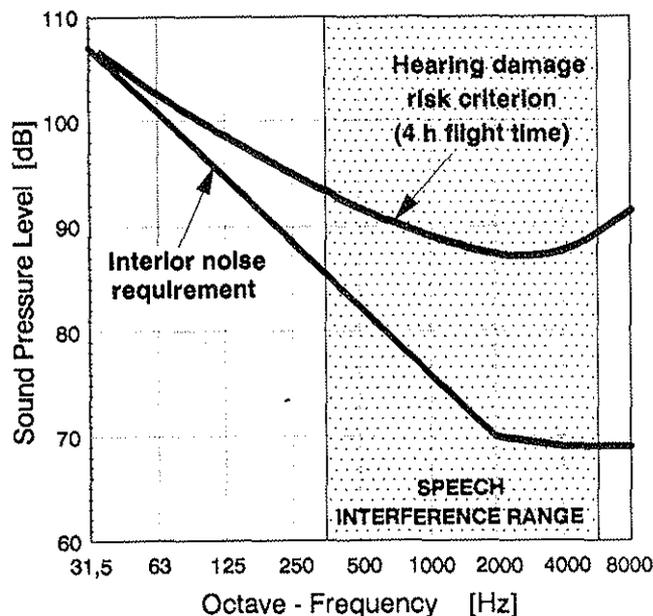
Figure 1: Definition of the Standard Interior Noise Requirement
