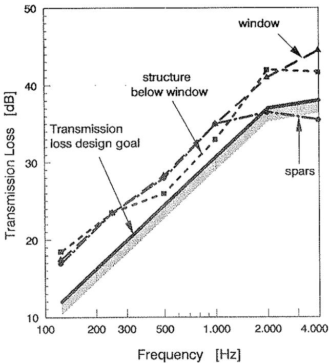
Figure 6: Transmission Loss Measurements of the BO 108 Cabin Door After Improvement
