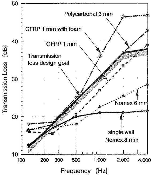
Figure 3: Transmission Loss of Different Double Wall Systems
