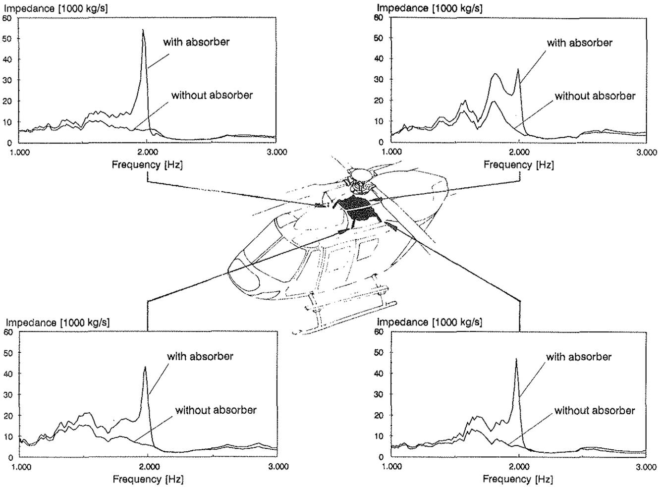
Figure 20: Impedance Measurements of the Four Vertical Gearbox Levers With and Without Absorbers
