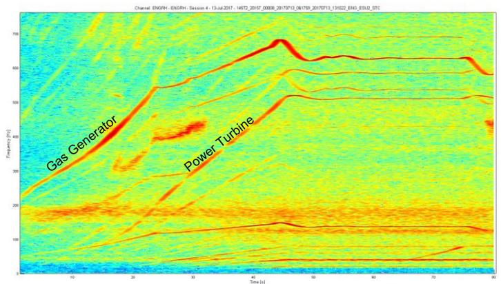
Figure 4 - Time-Frequency diagram of an engine run-up
