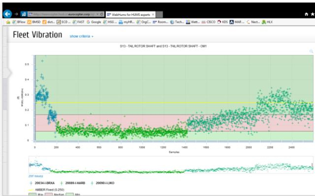
Figure 18 – Airbus Helicopter webHEALTH online service for expert analysis of drive train vibration
