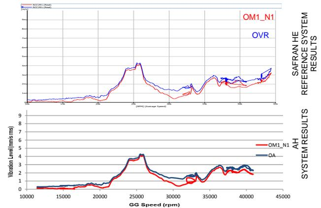
Figure 12 – Ground Test Results: comparison of AH system processing (top) and SAFRAN HE reference system (bottom) results for an engine run up
