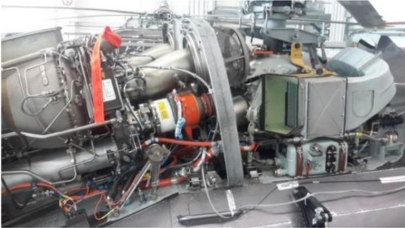
Figure 10 – Instrumented ARRIEL2E engine during qualification campaign
