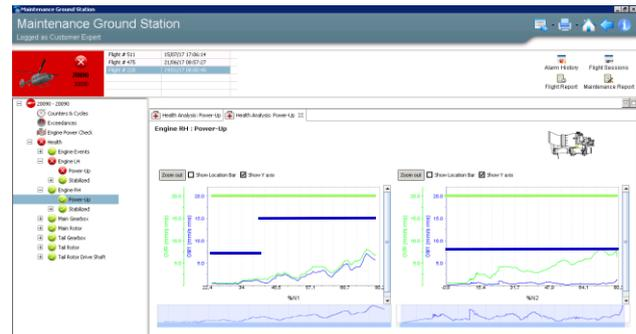
Figure 15 – Airbus Helicopters Maintenance Groundstation Engine Vibration Monitoring (engine run up)
