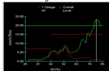
Figure 21 – Overall level alarm during engine power up acquisitions
