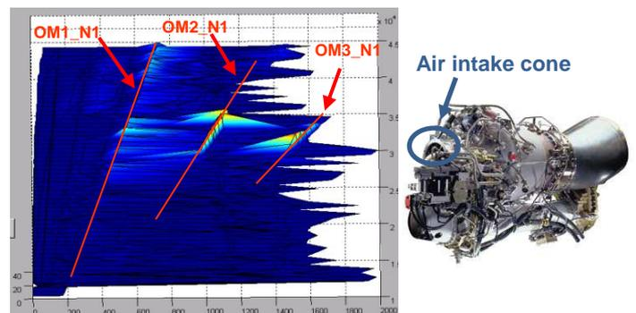
Figure 20 – Spectral analysis based on the raw data recorded by the EVM function
