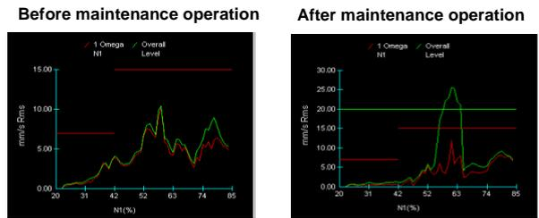
Figure 19 – Engine vibration curves recorded before and after a maintenance operation
