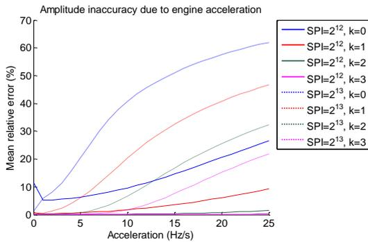
Figure 7 – Engine vibration amplitude accuracy during engine acceleration as function of samples per interval (SPI) and number of adjacent samples
