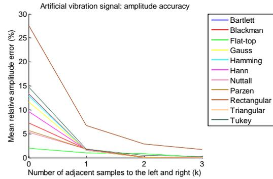
Figure 8 – Engine vibration amplitude accuracy during engine acceleration as function of Window type and number of adjacent samples
