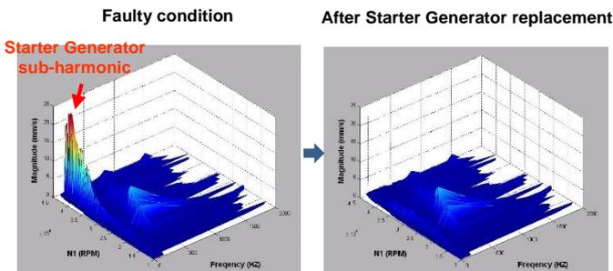
Figure 23 – Spectral analysis with Safran Helicopter Engines dedicated vibration tool
