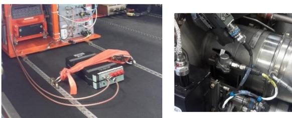
Figure 11 – Safran Helicopter Engines reference system installed in the BK117 D-2 cabin compartment during flight test campaign
