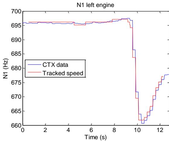
Figure 6 – Engine speed tracked using vibration data
