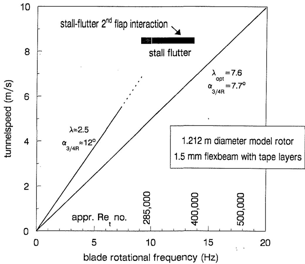
Fig. 2: Instability diagram denoting 2<sup>nd</sup> flap interaction range
