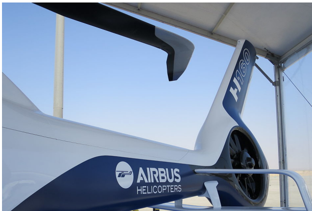
Figure 1: Fore-aft swept blade tip and tail section of the H160 helicopter 18 .
